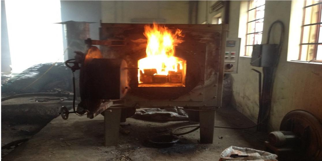
**Fig. 3:** Burning specimen inside furnace after expiration of 1-hour fire exposure
