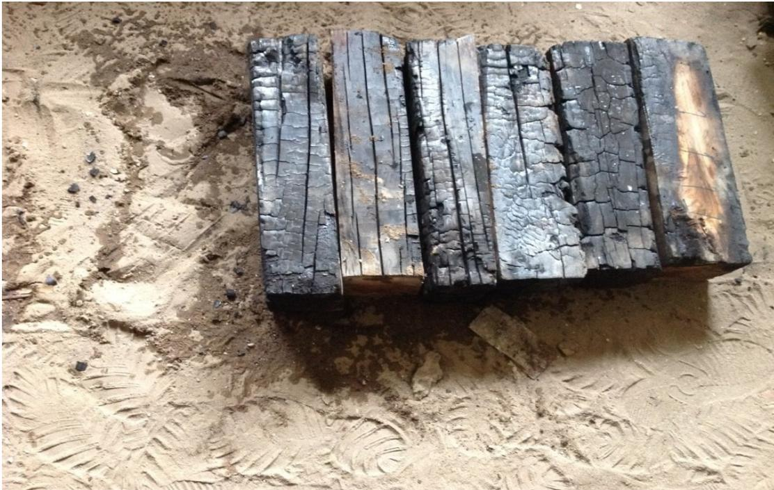
**Fig. 4:** Charred wood after 1-hour fire exposure
