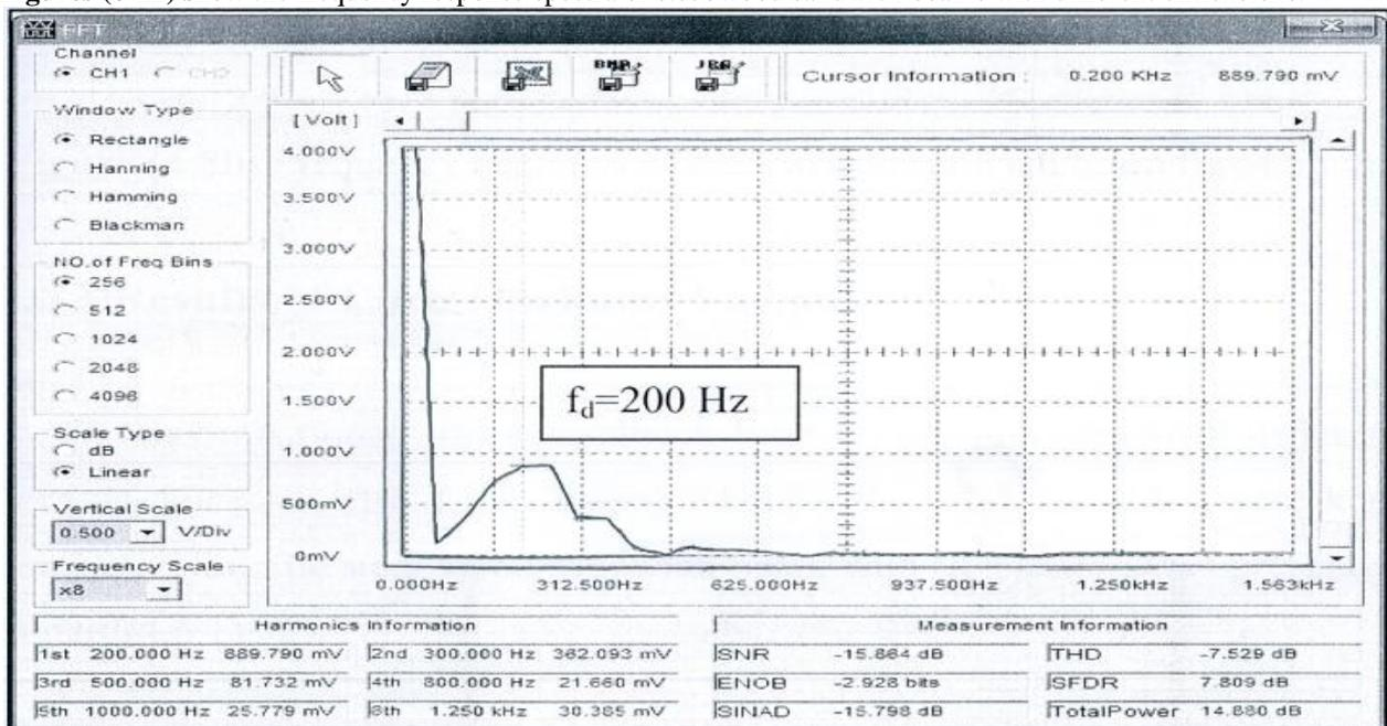
**Figure 6:** Frequency Response Spectrum of Steel/Wood Sandwich Beam ( $h_f = 1.5\text{mm}$ ,  $h_c = 10\text{mm}$ ,  $B = 25\text{mm}$ , and  $L = 180\text{mm}$ )
