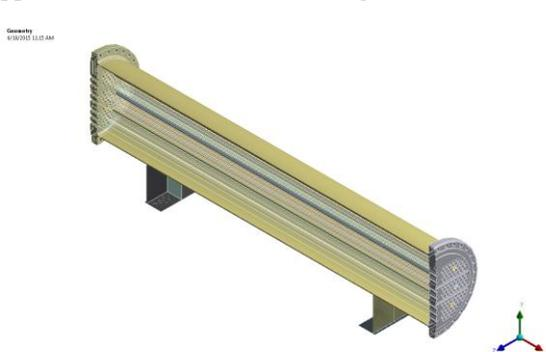
Fig. 4: FE model with beams- section view
