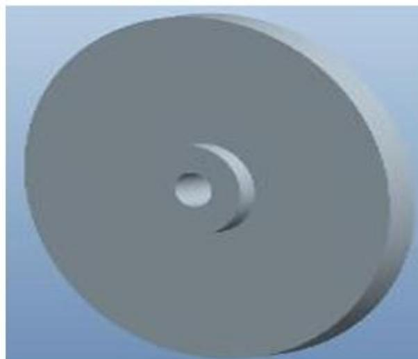
**Fig.4. Drafting & Modeling of Solid Disk Flywheel**
