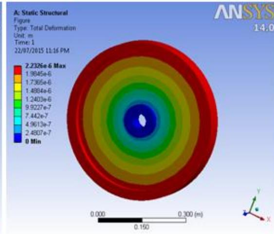
Fig.8. Deflection in Optimal Solid
