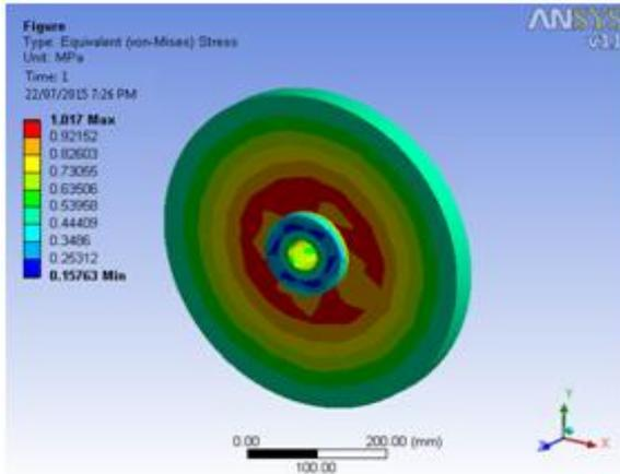
Fig.5. EquiVon Mises In Solid Flywheel
