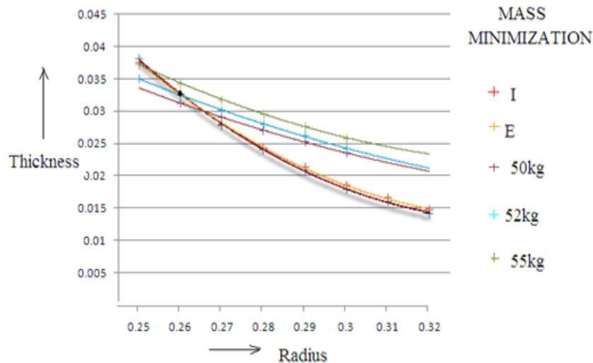
Fig.1. Graphical Representation of Mass Minimization of Solid Disk Flywheel
