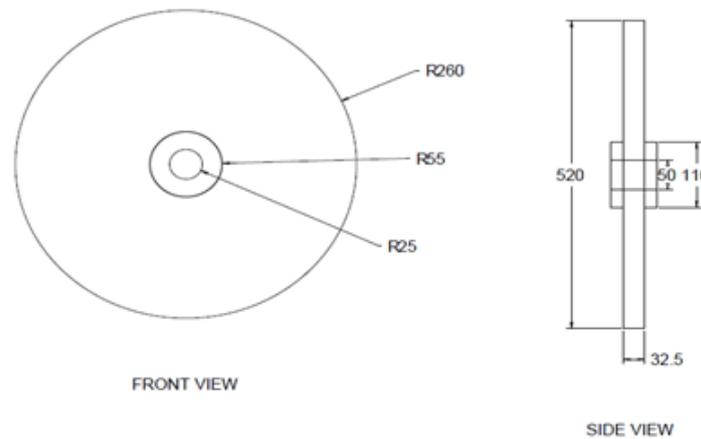
Fig.2. Optimal Solid Flywheel
