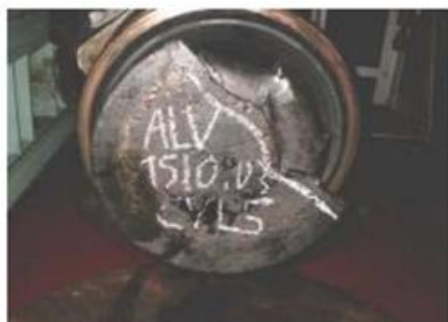
Fig2.1 Catastrophic failure of a repaired valve spindle (RTA 72)
