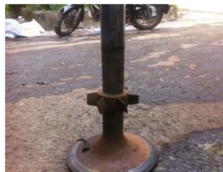
Fig1.2 Actual photo of spindle with rotor wings showing uniform wear rate
