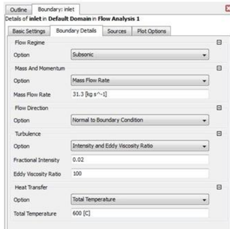
Fig3.5 Inlet details
