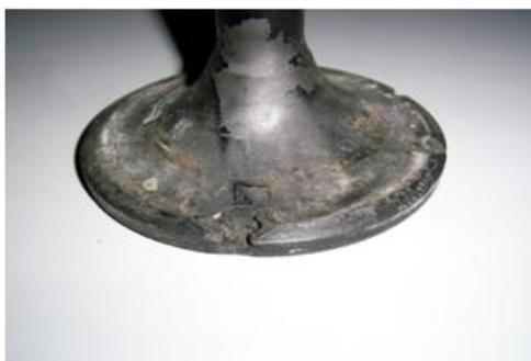
Fig1.1 Excessive damage on one section of the spindle
