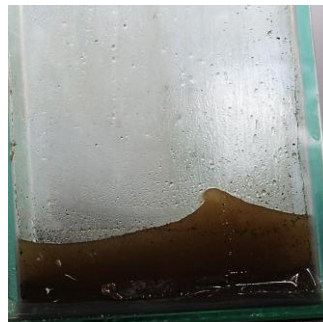
Fig 2.5 Density Variable TLD (consisting of sand and water)
