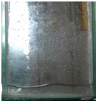
Fig 2.3 Traditional TLD (consisting of water as liquid)
