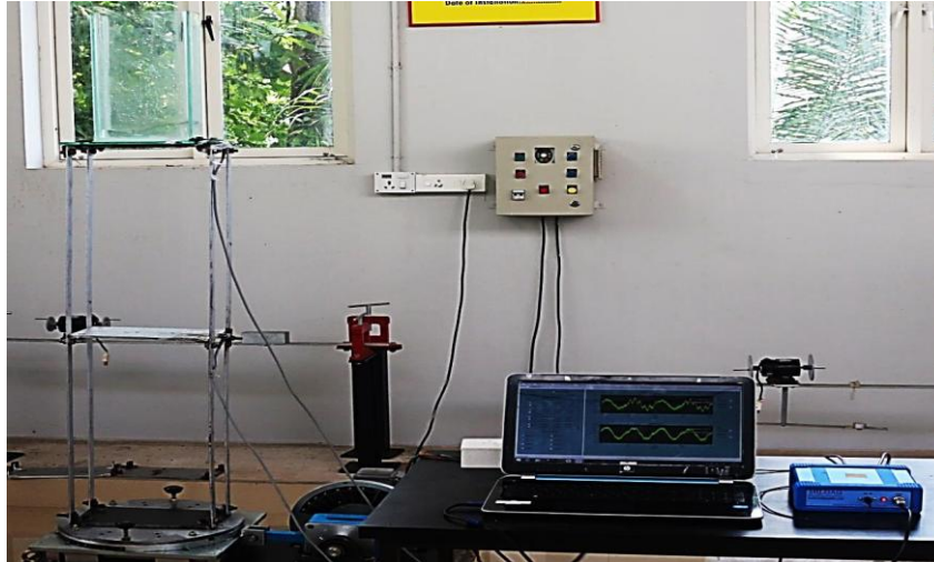
Fig 2.2 Experimental Setup of the Structural Model Damped with TLD
