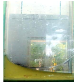
Fig 2.4 Viscous TLD (consisting of oil)
