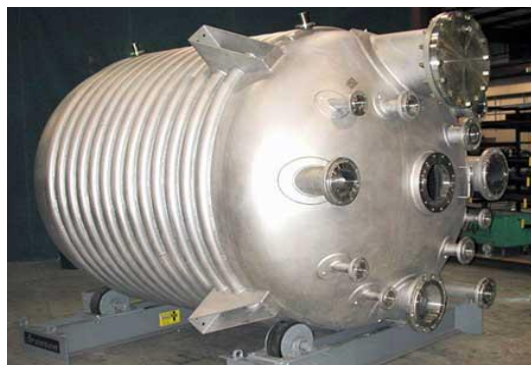
Fig.1 Pictorial view of pressure vessel
