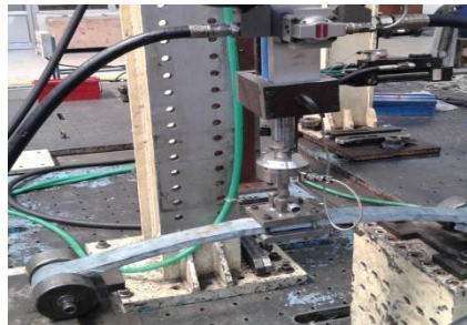
Figure 2 . Servo hydraulic Actuator Test Rig
