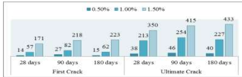
Fig. 5 Percentage Improvement In First Crack and Ultimate Crack Strength of High Volumes of Slag Fibre Concrete over High Volumes of Slag Concrete (w/b=0.36)
