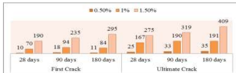
Fig. 6 Percentage Improvement In First Ultimate Crack Strength of High Volumes of Slag Fibre Concrete over High Volumes of Slag Concrete (w/b=0.27)
