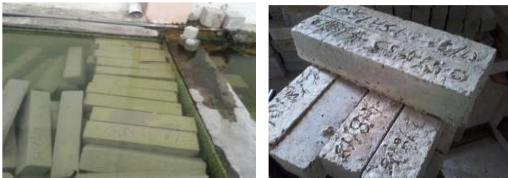
Fig. 8 Specimens of HVSC before and after curing
