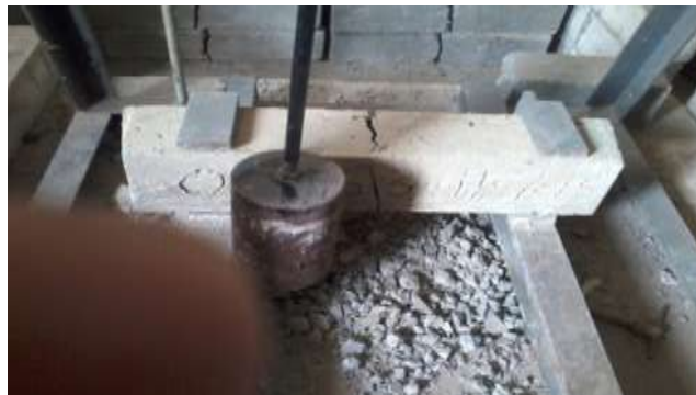
Fig.9 Failure at Ultimate Crack of Specimen of HVSC
