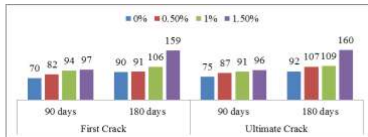
Fig.3 Percentage Improvement in First Crack and Ultimate Strength of High Volumes of Slag Concrete With & Without Fibres over 28 Days Impact Strength (w/b=0.27)
