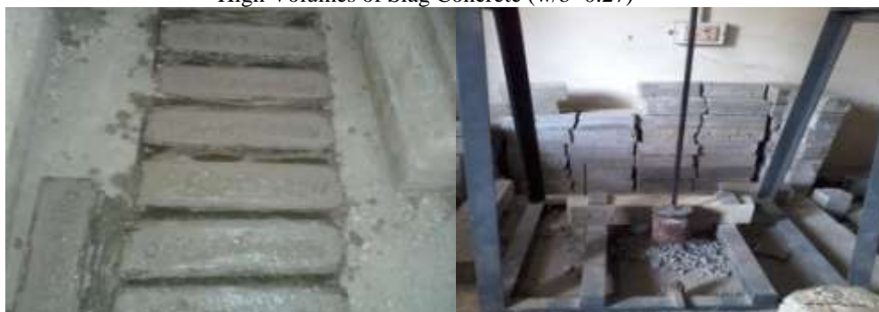
Fig. 7 Casting and Testing of Specimens of HVSC with Steel Fibres
