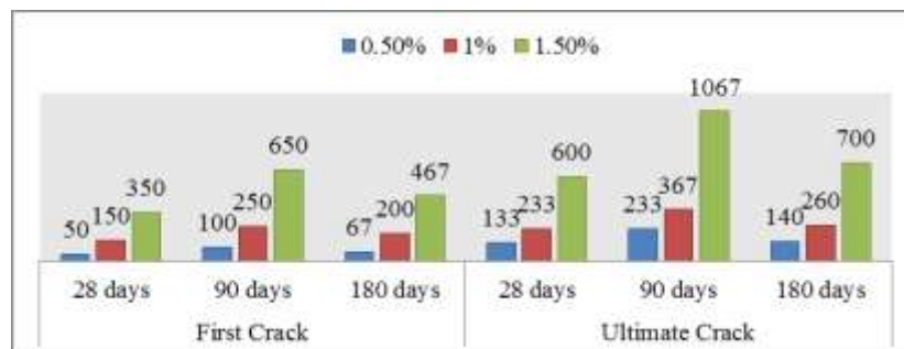
Fig. 4 Percentage Improvement in First Crack and Ultimate Crack Strength of High Volumes of Slag Fibre Concrete over High Volumes of Slag Concrete (w/b=0.55)
