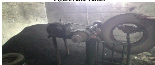
Fig 1. Formation of Rubber Shreds from the Cutting Machine
