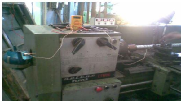
Fig. 3 Setup for temperature measurement using thermocouple
