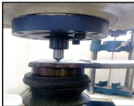
Fig 5.2 Figure of the Variation of hardness in fusion zone and heat affected zone on Mild steel
