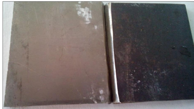
Fig 4.7 Figure of original Specimen of work piece with V Groove
