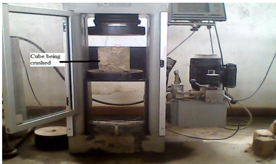
Figure 1: Compression machine used for the cube crushing test
