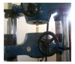
Specimen during testing Below figure shows the specimen after tensile testing. It shows that it has been broke into two parts.
