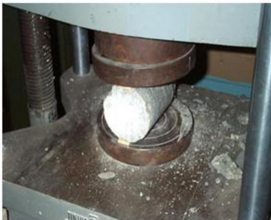
Fig.3 Split Tensile testing
