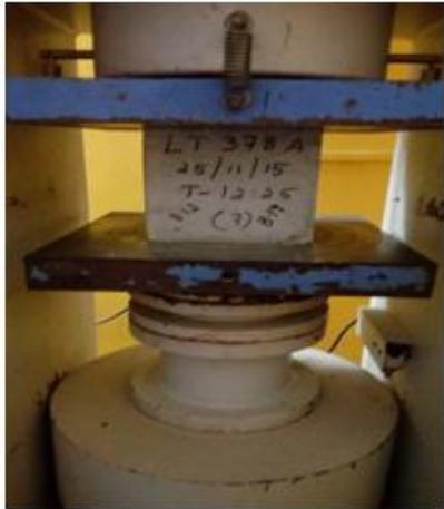
Fig.3 Compression testing
