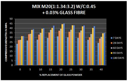
Mix M20(1:1.34:3.2) w/c:0.45 replace by glass powder + 0.03% glass fibre
