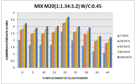
Mix M20(1:1.34:3.2) w/c:0.45replace by glass powder + 0.03% glass fibre
