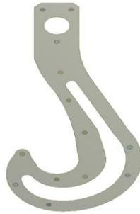
Fig13: Design for Iteration 9 with changed rivet positions and cut
