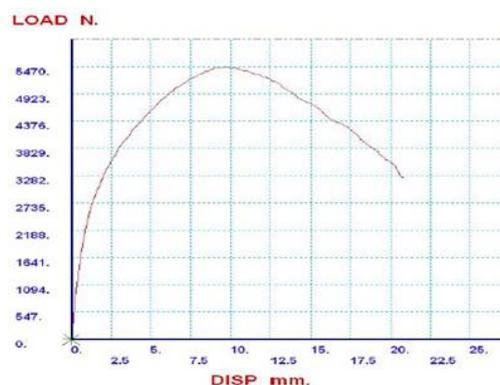
Fig25. Load-Displacement relation of laminated hook
