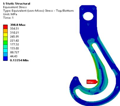
Fig 14: Von mises plot for Iteration 8
