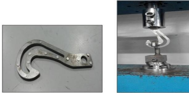
Fig26. laminated hook before tensile testing
