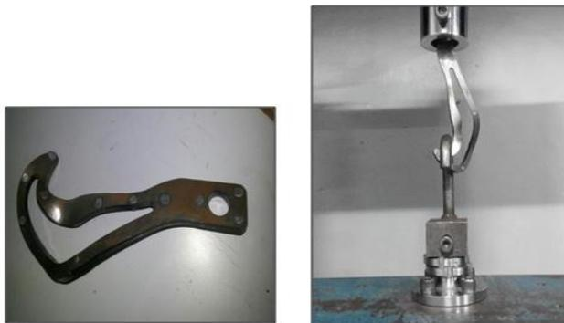
Fig27] Laminated hook after tensile testing
