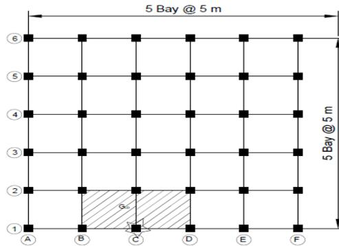
Fig.3.3 Exterior Column Removal Location
