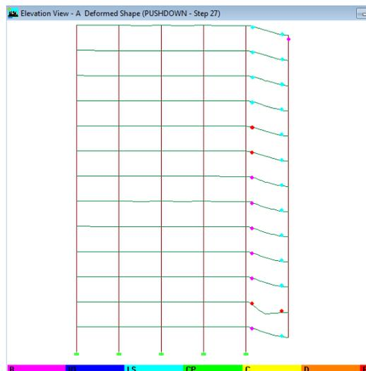
Fig.3.8 Hinge formation for elevation a corner column removal case
