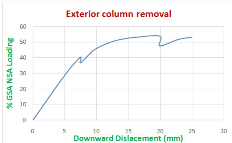
Fig.3.9 % GSA loading vs Monitored deflection at Exterior column removed
