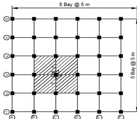
Fig.3.5 Interior column removal case
