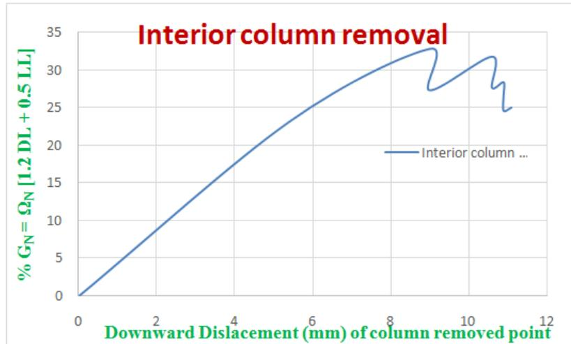
Fig.3.11 % GSA loading vs. Monitored deflection at Interior column removed
