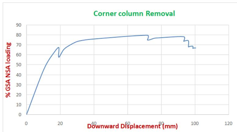
Fig.3.7 % GSA loading vs Monitored deflection at column removed point
