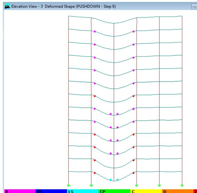
Fig.3.12 Hinge formation for elevation 3 Interior column removal
