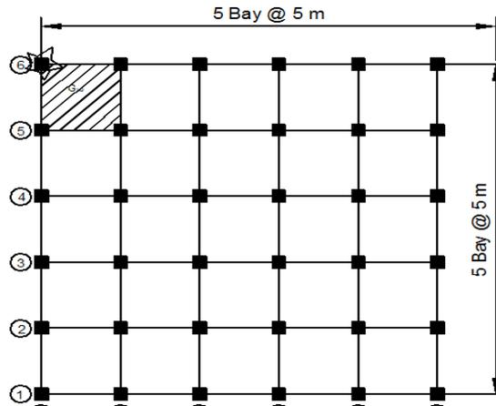
Fig 3.1: Corner Column Removal
