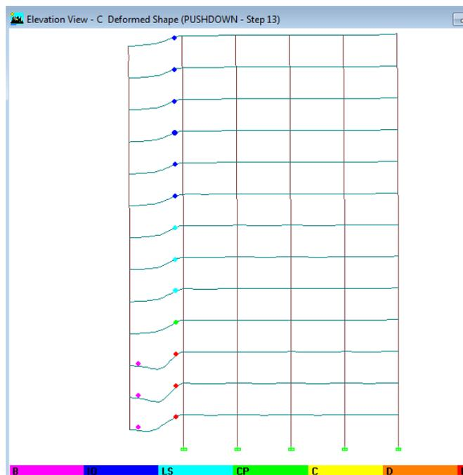
Fig.3.10 Hinge formation for elevation C exterior column removal
