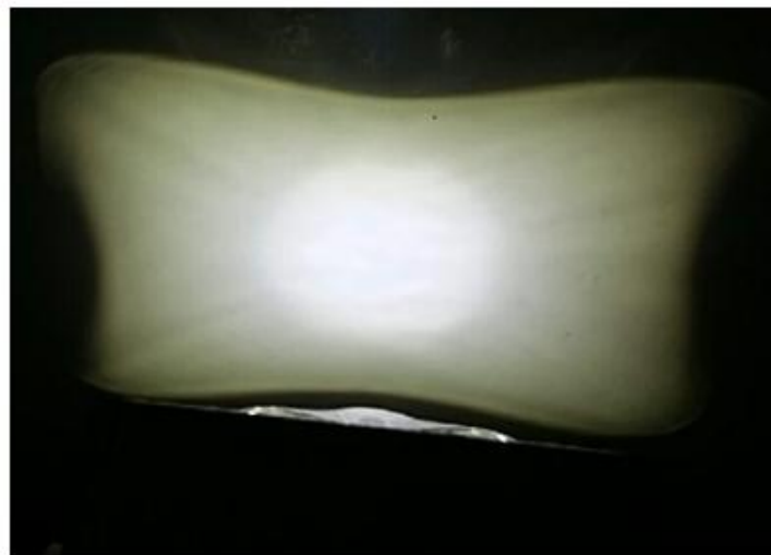
Fig. 13 Illumination with discrete uniformities for Case 1 by experiment.
