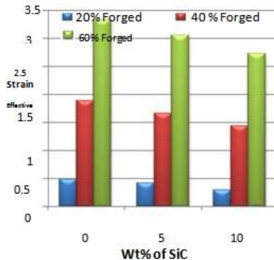
Fig. 13 Comparison of forging effect and wt% of SiC on the Effective Strain of Al-SiC
