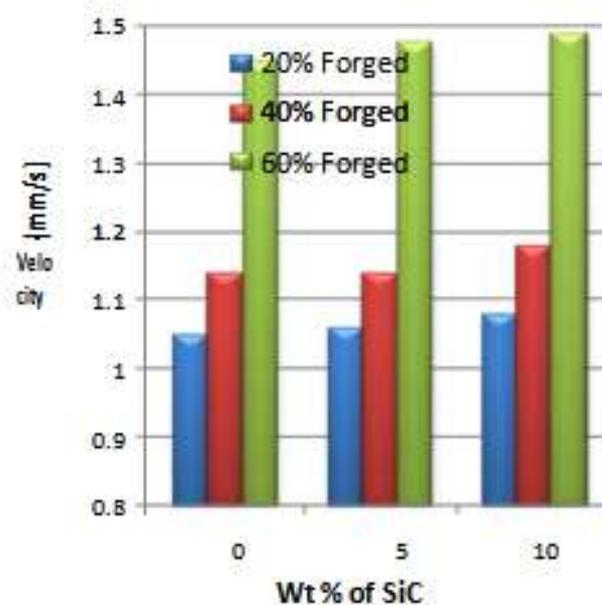
Fig 13 Comparison of forging effect and wt% of SiC on the damage of Al-SiC MMCs
