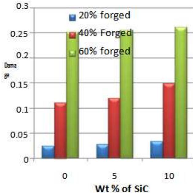
Fig 12 Comparison of forging effect and wt% of SiC on the damage of Al-SiC MMCs
