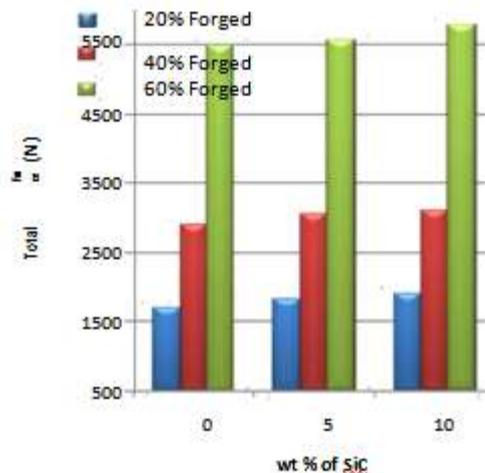
Fig 14 Comparison of forging effect and wt% of SiC on the total force of Al-SiC composite
