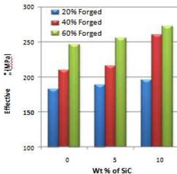
Fig. 12 Comparison of forging effect and wt % of SiC on the effective stress of Al-SiC
