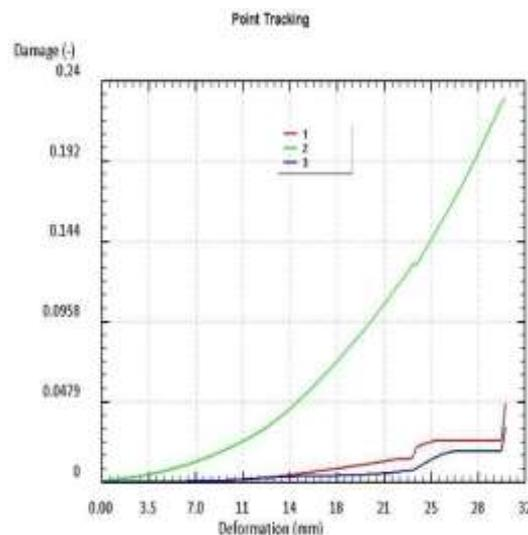
Fig. 7 Variation of damage vs. deformation along the point tracking
