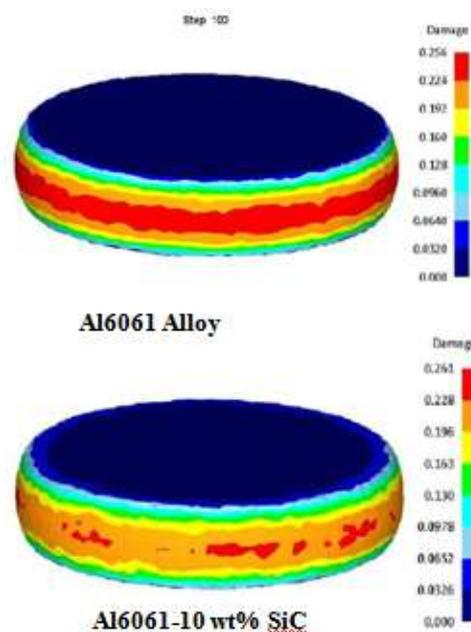
**Fig. 5** Variation of damage in Deform-3d
