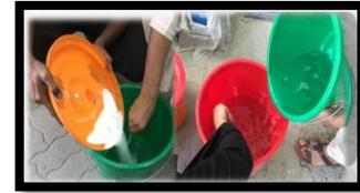
Fig.3 Mixing of Alkaline Solution (8M)
