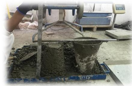
**Fig.9 Slump Test for GPC**
