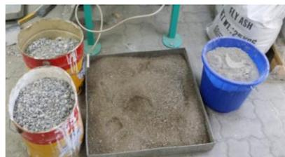
Fig.5 Fine aggregate, coarse aggregate and flyash
