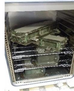
Fig.15 Prisms in Heat Chamber
