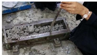
**Fig.11Casting of Prism**
