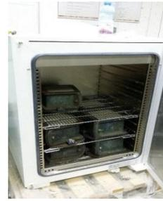
Fig.13 Cubes in Heat Chamber
