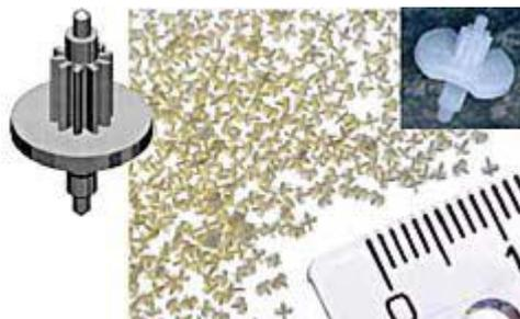
**Fig 3:** Plastic gear for watches using micro gear die
