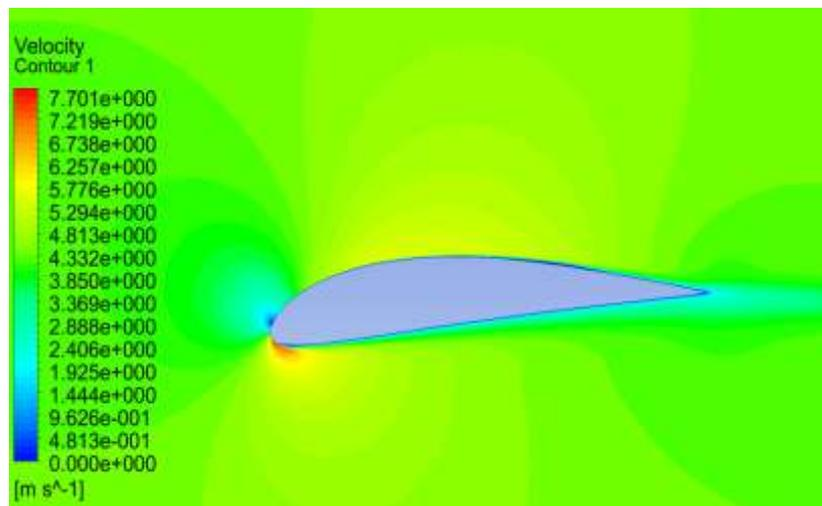
Figure 4: Contours of velocity magnitude at -5 degrees of angle of attack
