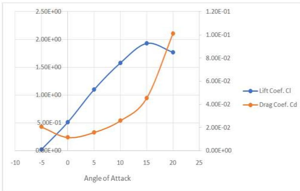
Figure 10: Curve of Lift & Drag Coefficients vs. Angle of Attack
