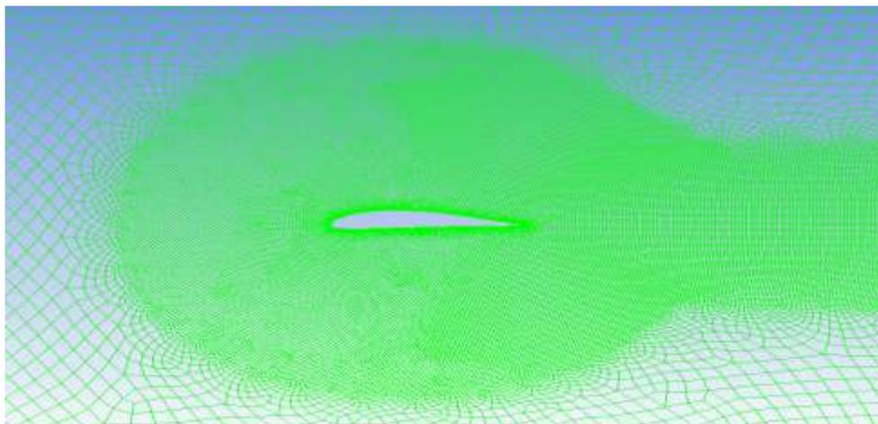
Figure 3: Mesh of the computational domain
