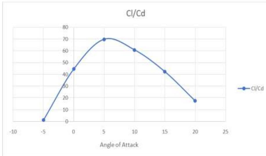
**Figure 11:** Curve of Lift to Drag Coefficients vs. Angle of Attack
