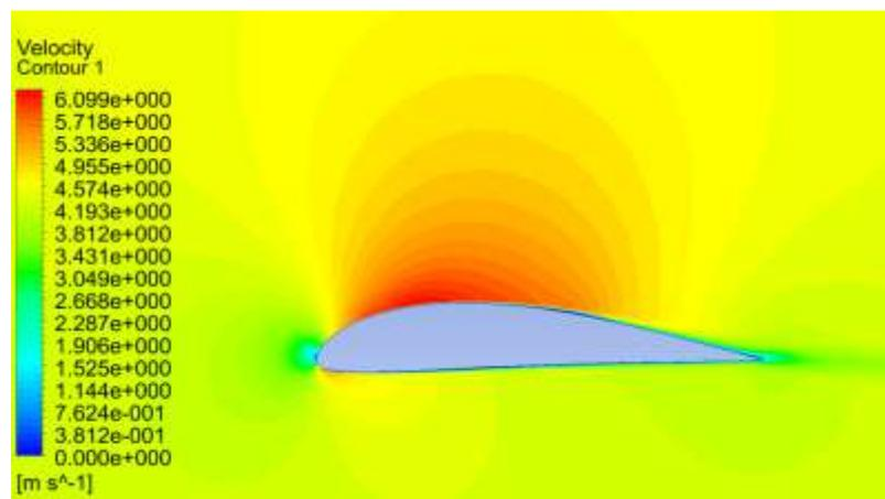
Figure 5: Contours of velocity magnitude at 0 degrees of angle of attack
