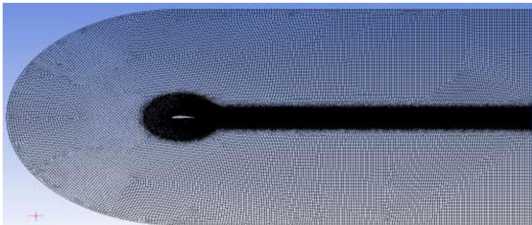
Figure 2: Completed Mesh
