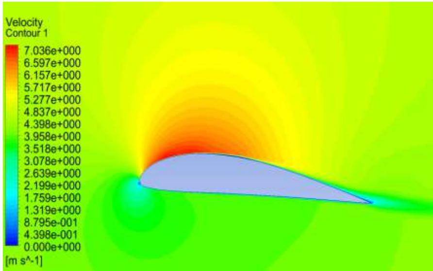
Figure 6: Contours of velocity magnitude at 5 degrees of angle of attack
