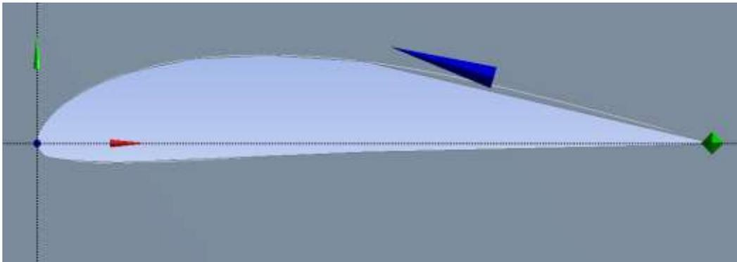
Figure 1: Geometry of GOE 387 Airfoil
