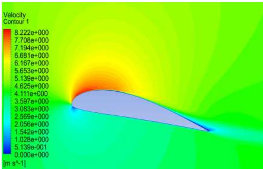
Figure 7: Contours of velocity magnitude at 10 degrees of angle of attack
