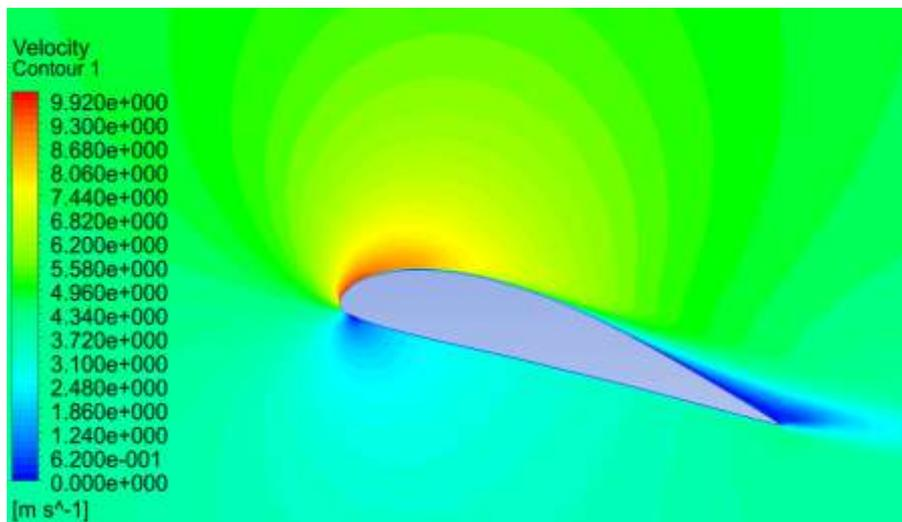
Figure 8: Contours of velocity magnitude at 15 degrees of angle of attack
