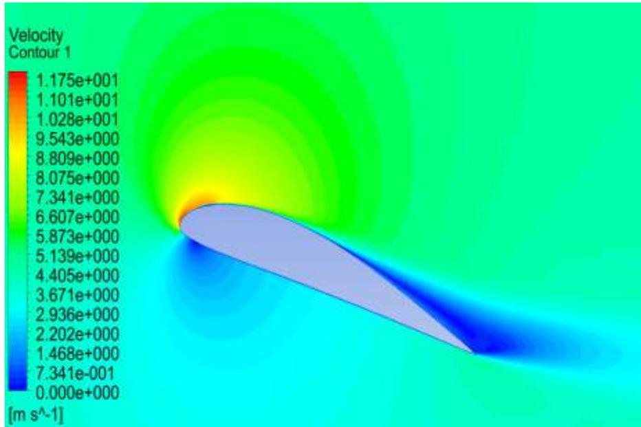
Figure 9: Contours of velocity magnitude at 20 degrees of angle of attack
