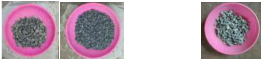
Local coarse aggregates (20mm and 12.5mm down size) GMW coarse aggregates (20mm down size)
