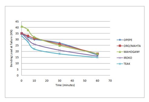
Fig. 6: Bending Load at failure - Time curve
