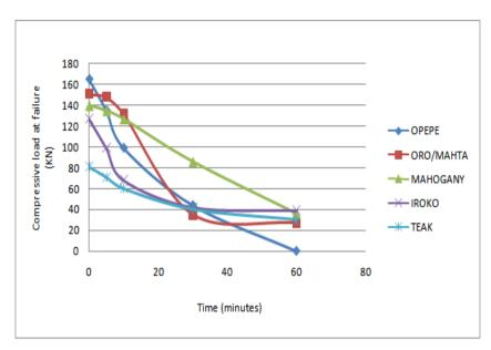
Fig. 4: Compressive load at failure - Time
