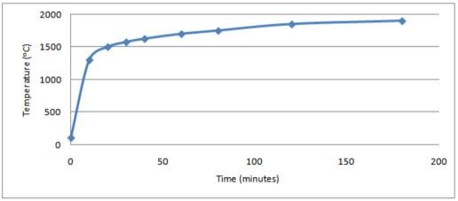
Fig. 1: ASTM Standard Temperature - Time curve for Fire Tests (Source: Schaffer, 1967)
