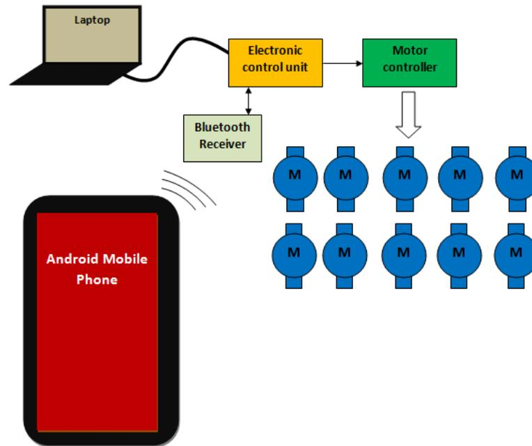
Figure 1 Schematic Diagram of MMT CNC
