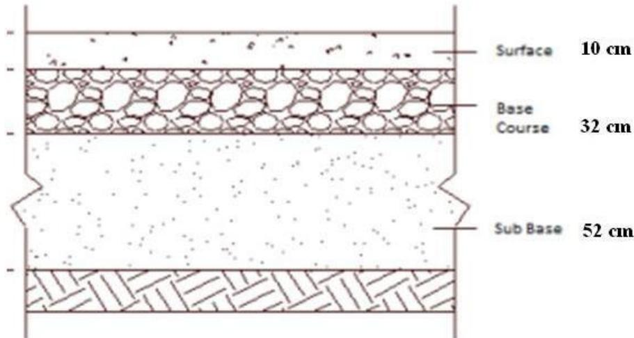
**Figure 5.** Pavement Thickness for  $PCN \geq 51 FDXT$
