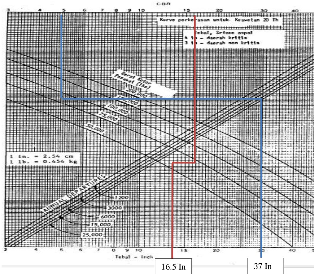
Figure 4. The thickness of pavement for aircraft plan B737-800
