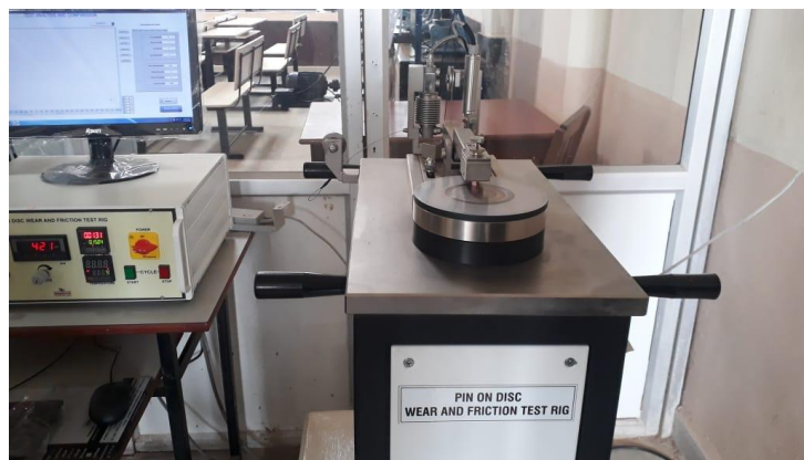
Figure 4 Pin-On-Disc Machine & Data Acquisition
