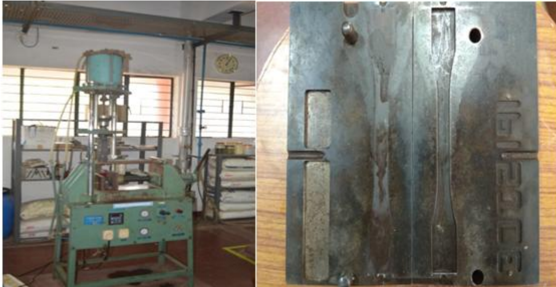
Figure 3 Injection moulding machine with mould cavity
