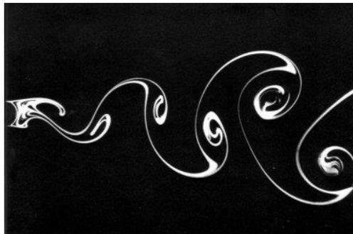
Figure 4. Streets of Von Karman generated behind a cylinder, consisting of vortices separated alternately.
