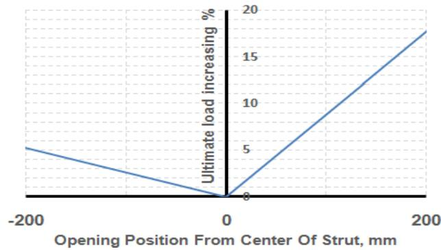
Fig. (11): Effect of Web Openings Position on CDB Ultimate Capacity.
