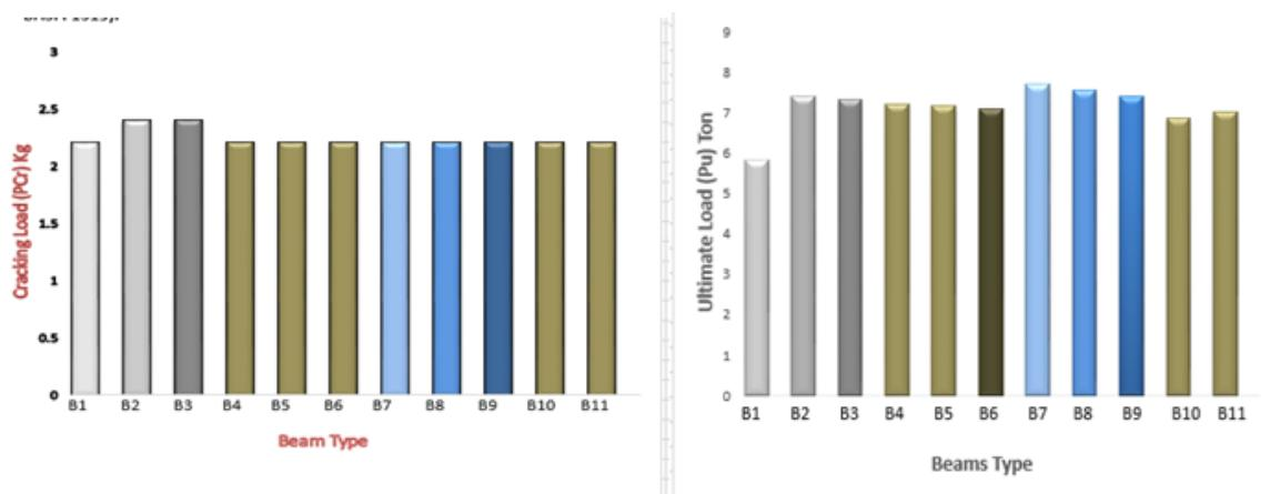
**Fig: ( 7 )**Cracking and Ultimate Loads for beams B1®,B2,B3,B4,B5,B6,B7,B8,B9,B10 &B11.
