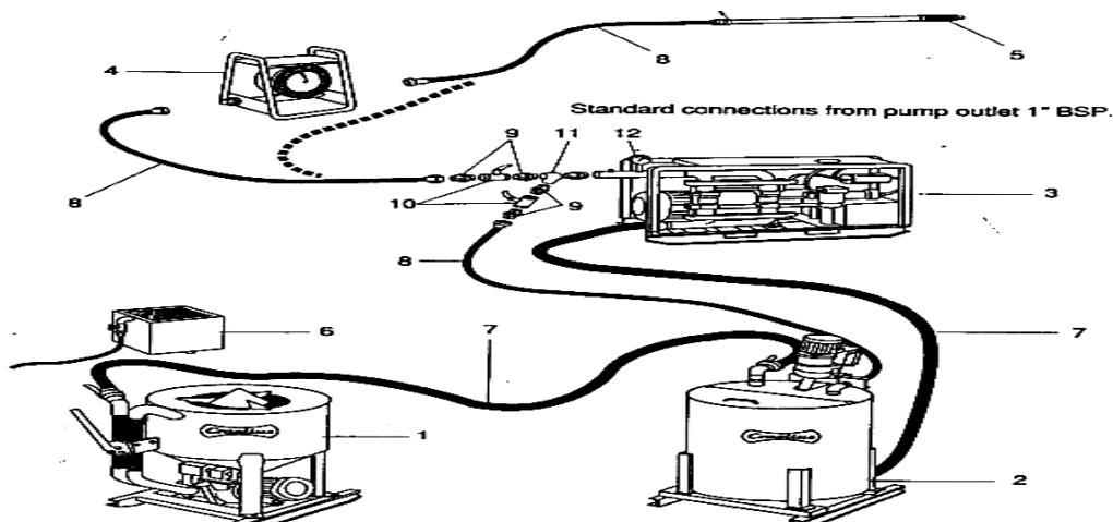
1-Mixer 2-Agitter 3-Pump 4-Recorder 5-Packers 6-Measuring tank 7-Mixer hose 8-Delivery
