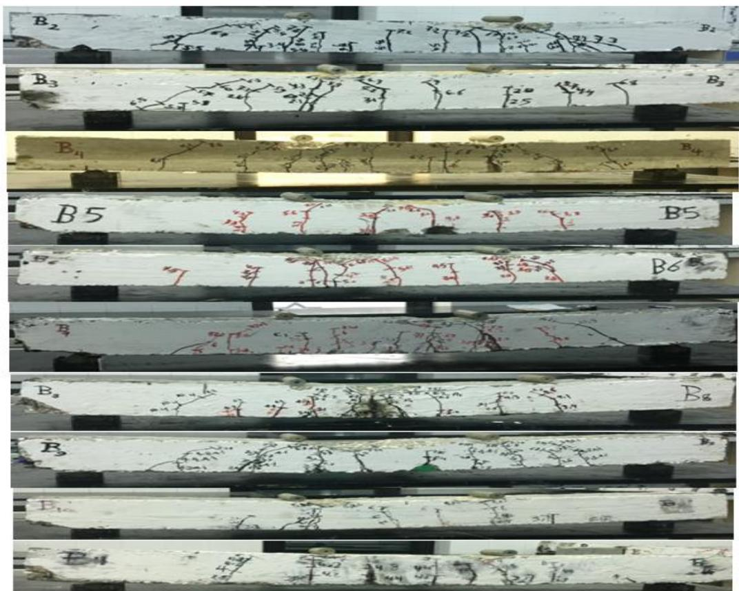
Fig: (6) Pattern of crack of beams B1®,B2,B3,B4,B5,B6,B7,B8,B9,B10 &B11.
