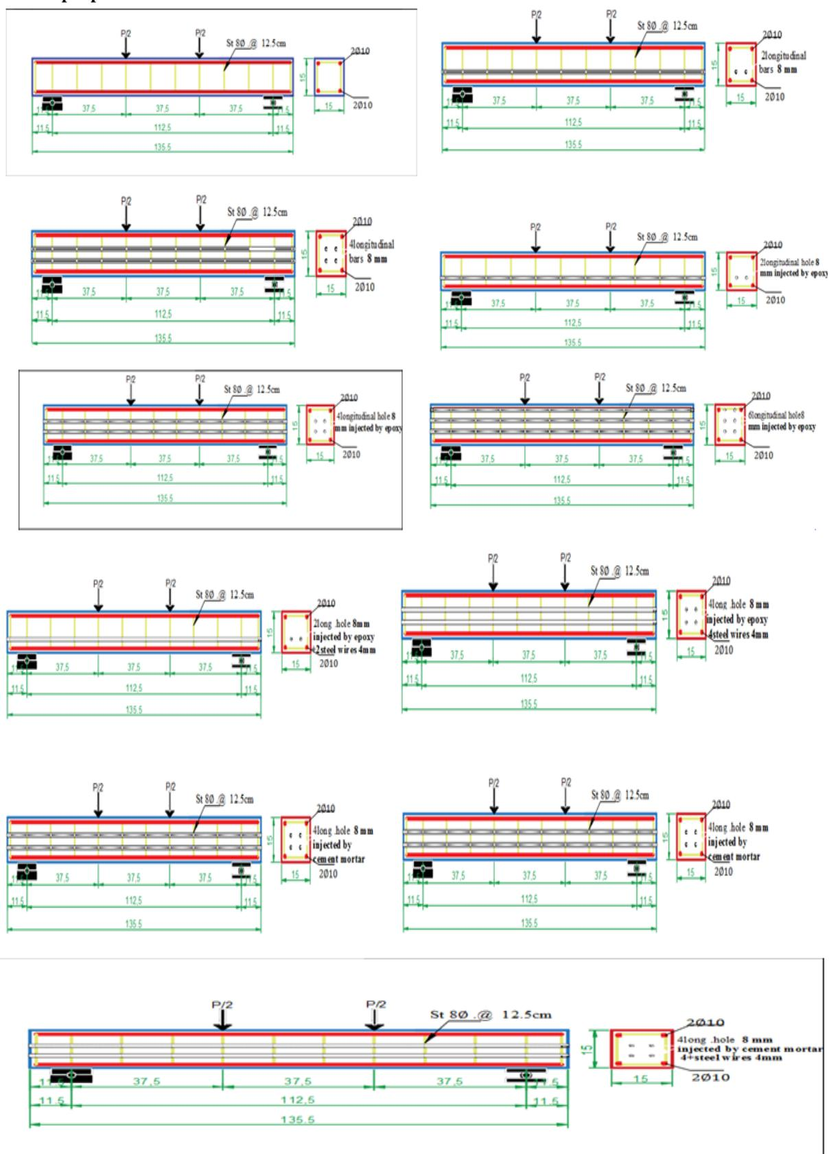
Fig.(2).Details of beams B1®,B2,B3,B4,B5,B6,B7.,B8.,B9.,B10.,&B11.
