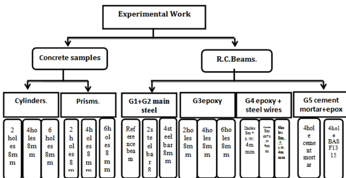
Fig. (1): The Experimental Work Program.
