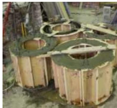
**Photo (3):** Concrete casting of pipes.
