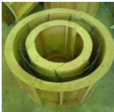
**Photo (2):** Wooden mould of pipes.
