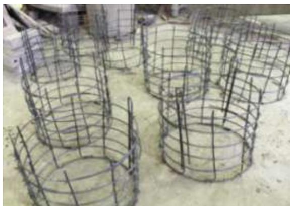
**Photo (1):**The typical reinforcement of the pipes.
