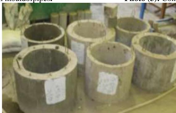
**Photo (4):** Curing of pipes.
