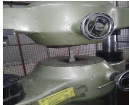
**Fig 3** Process setup for tensile test
