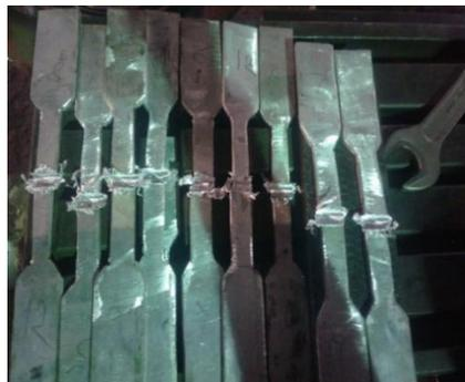
**Fig 2** Tensile test specimen
