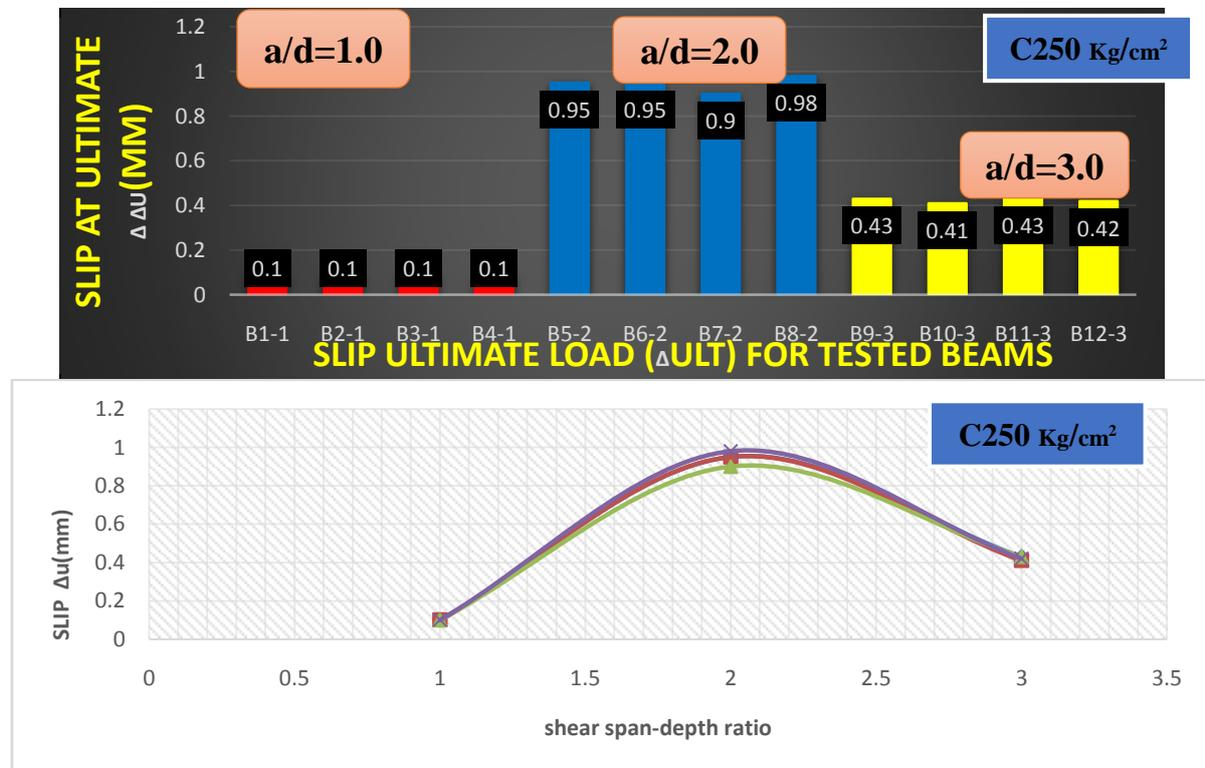
Fig (14). Slip at cracking loads ( $\Delta_{cr}$ .mm) and Ultimate loads ( $\Delta_{u}$ .exp.) for beams B1-1-®, B2-1-STR, B3-1-REP, B4-1-STR&REP, group 1. ( $\frac{a}{d} = 1.0$ ).  $L=92.5$ CM. B5-2®, B6-2-STR, B7-2-REP., B8-2-STR&REP group 2. ( $\frac{a}{d} = 2.0$ ).  $L=117.5$ CM. B9-3®, B10-3-STR., & B11-3-REP & B12-3-STR&REP. group 3. ( $\frac{a}{d} = 3.0$ ).  $L=142.5$ CM.
