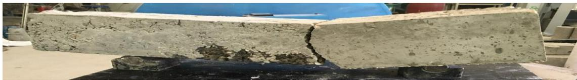
The initiation and propagation of the first crack for all beams observed in the bottom side of pure moment zone at mid span. Increasing the applied load gradually the formed cracks propagated upward and several new cracks observed in the tension zone, these started also from the bottom of concrete surface and propagated up to comp-zone.
