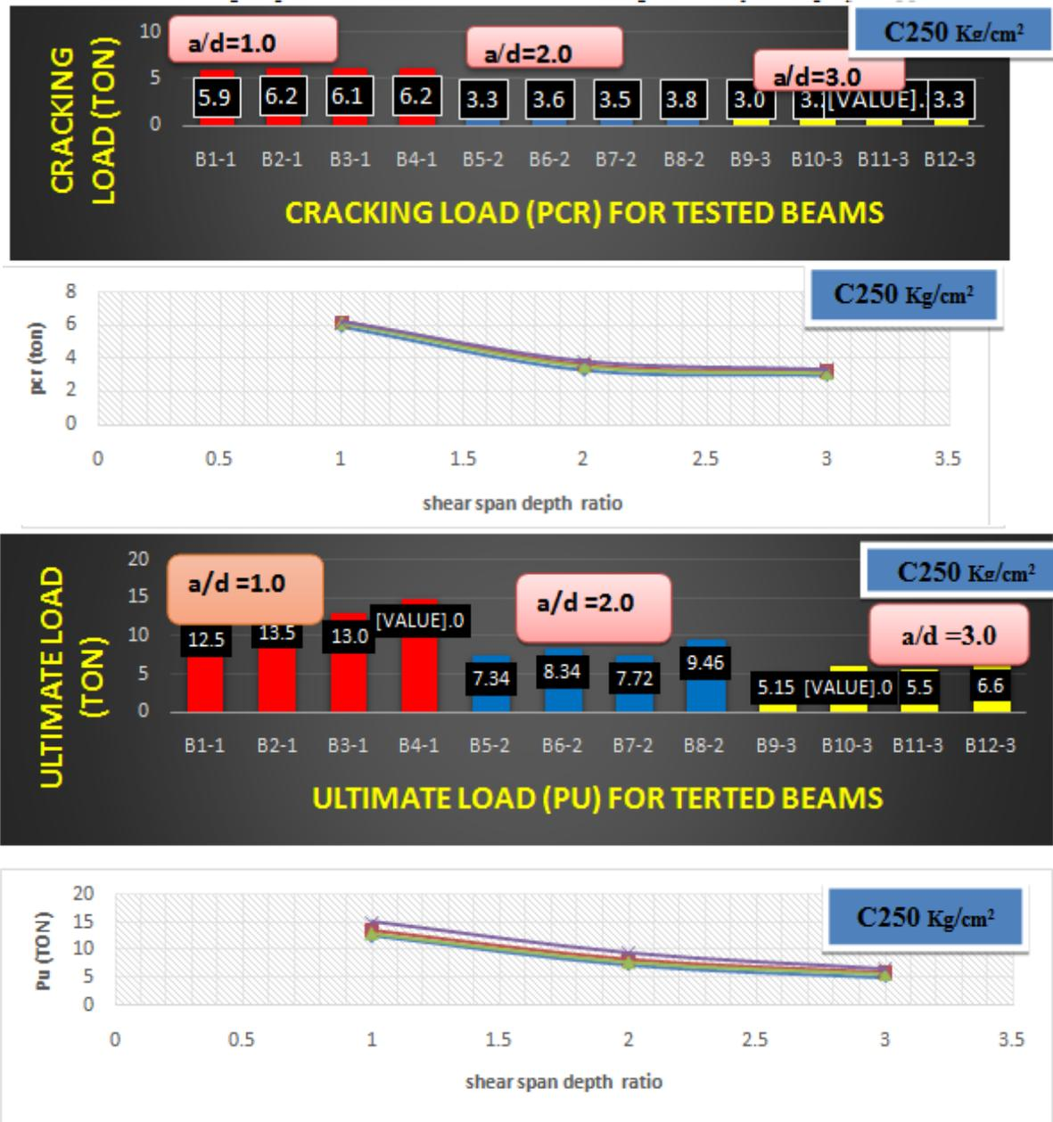
Fig: (9) Cracking and Ultimate Loads for beams
