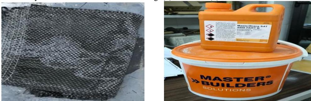
**Figure (4): CFRP sheets and Master Brace SAT 4500 Part A&B, BASFE**
