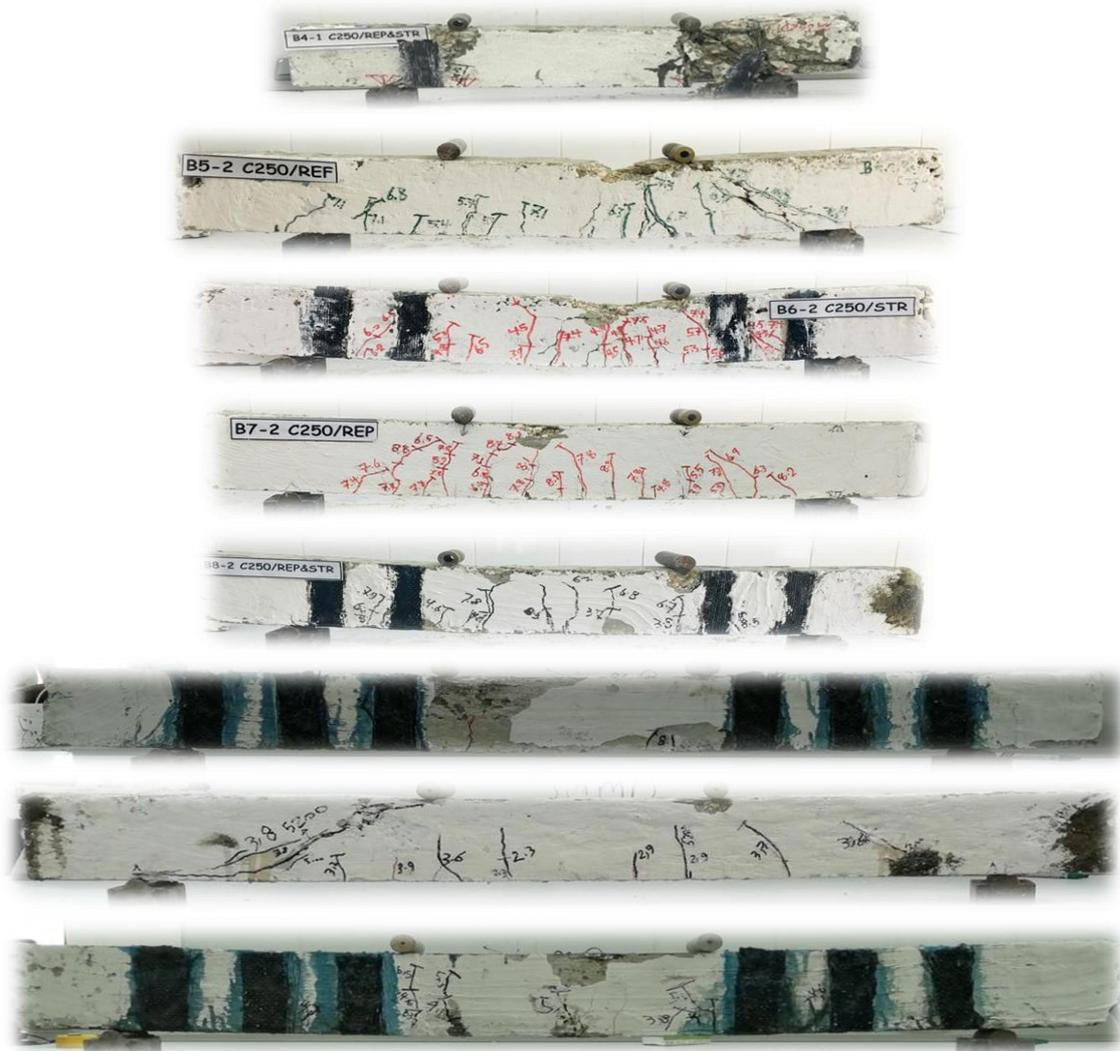
**Fig: (8)** Pattern of crack of beams
