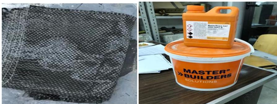
B, BASFE&Master Brace SAT 4500 Part A and Figure (4): CFRP sheets
