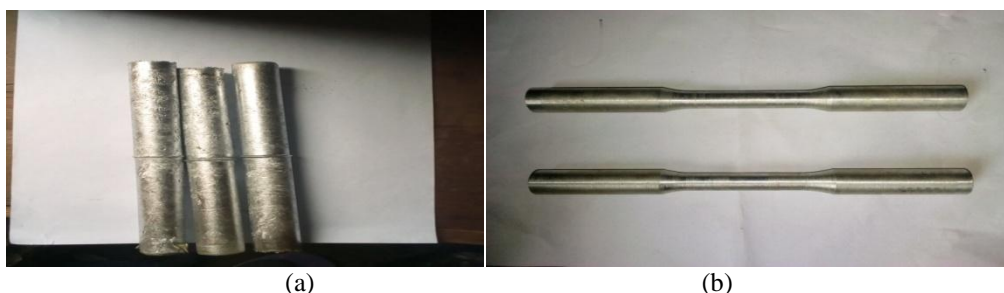
Plate V: (a) As cast tensile specimen and (b) Produced tensile strength test specimens
