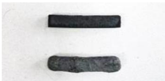
Fig. 5 Morphology of two samples after vacuum sintering and air sintering
