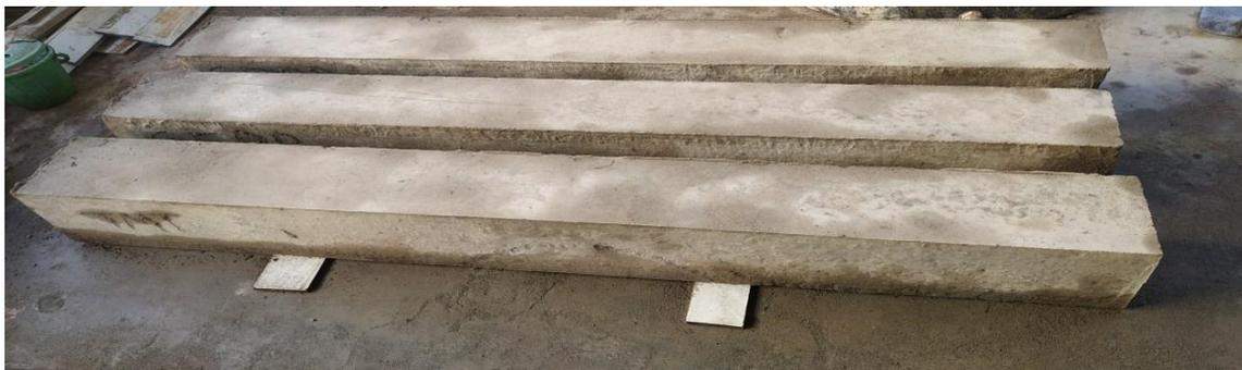
Fig.(6) Beam (B1, B2, and B3) specimens were constructed
