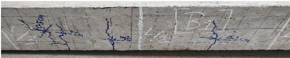
**Fig.(13)** The crack pattern of B1
