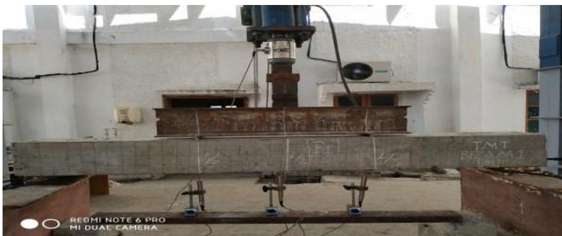
Fig.(12) Flexural loading setup
