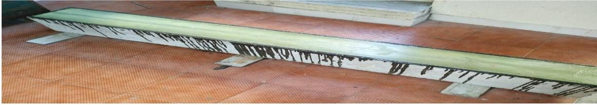
Fig.(10) Fiberglass epoxy flat strip was fixed on beam(B3)specimen
