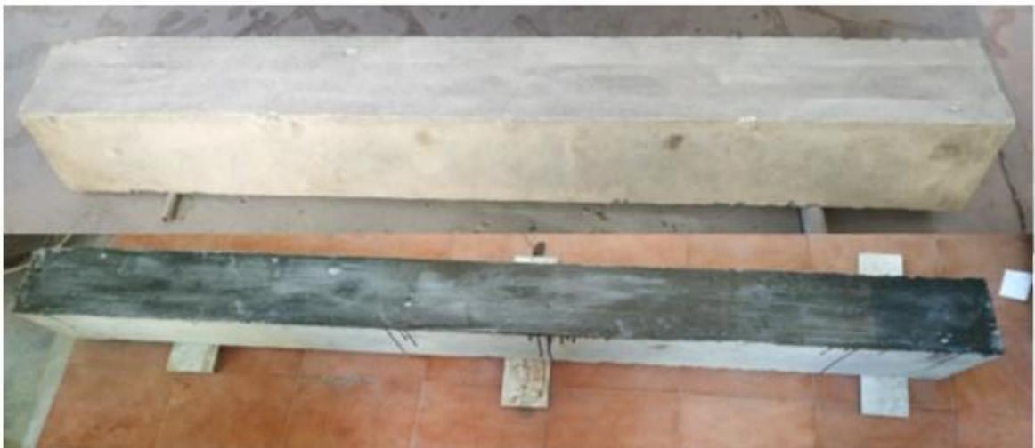
**Fig.(8)**The smoothed surface ofbeam(B3)specimenwere coatedwith epoxyresin
