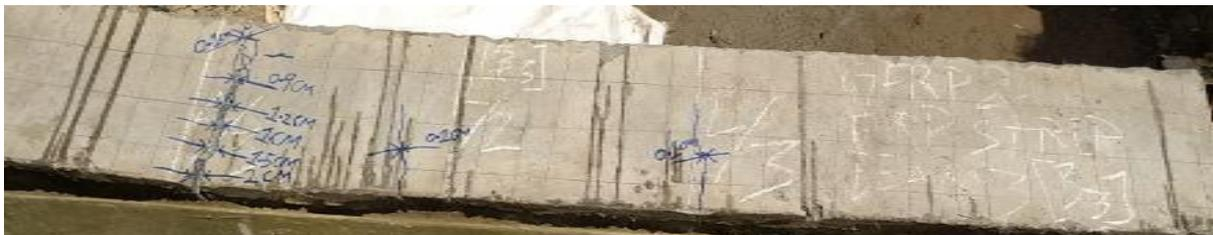
**Fig.(15)** The crack pattern of B3
