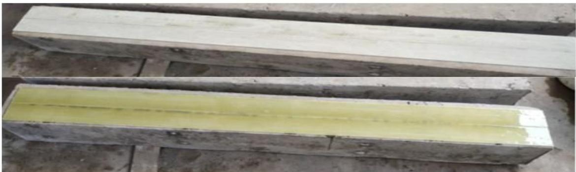
**Fig.(9)**The smoothed surface ofFiberglass epoxy flatstripwascoatedwith epoxyresin
