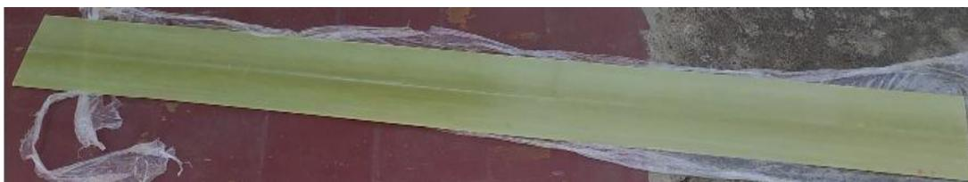
**Fig.(2)** Fiberglass epoxy flat strip
