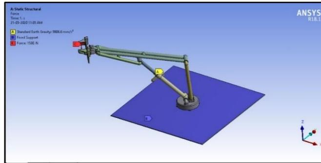
Figure 9: Application of load in Extended Configuration
