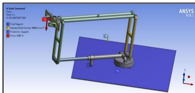
**Figure 8:** Application of load in Parallelogram Configuration
