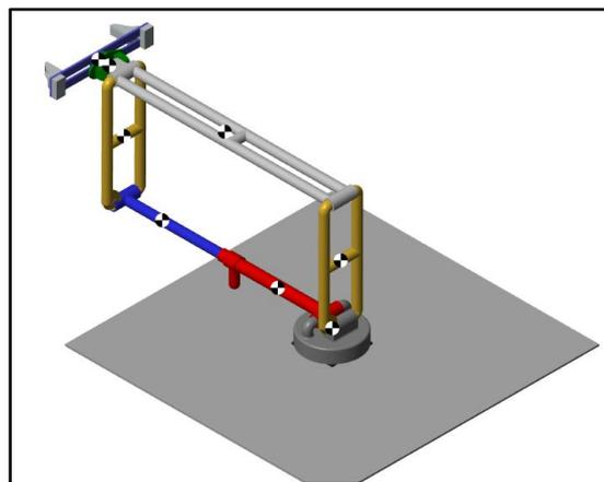
**Figure 1:** Isometric view of proposed robot design
