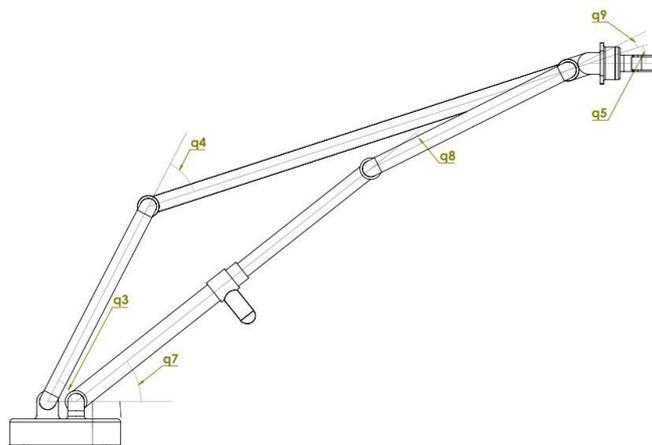
**Figure 7:** Parameters in Parallelogram extended configuration
