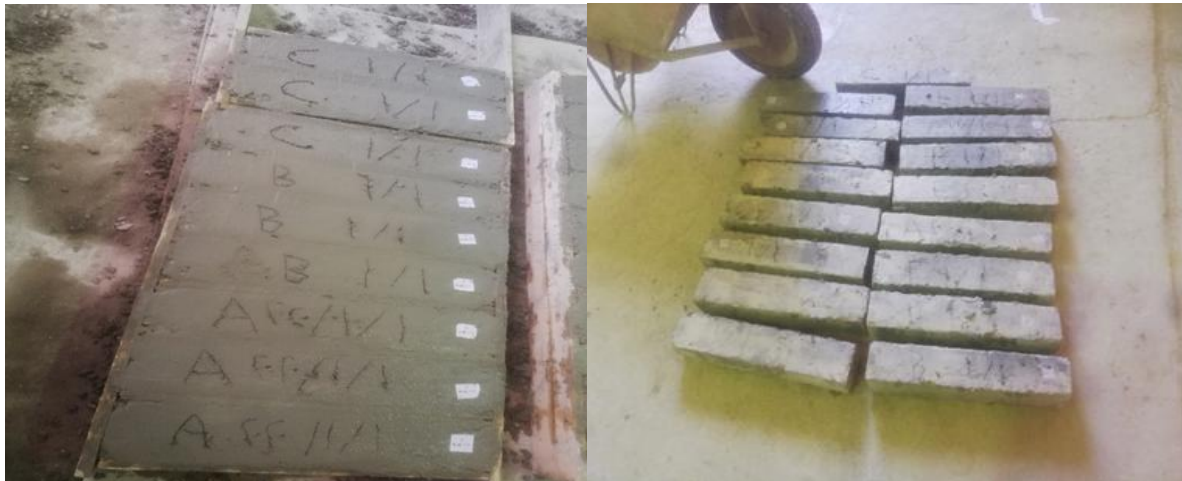
Fig. 10a: Beams (100 mm *100 mm*500mm) Fig.10b: Beams (100 mm *100 mm*500mm) during Casting.after Curing.
