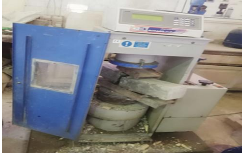
Fig. 13b: Beam (100 mm *100 mm*500mm) during Flexural Strength Test.
