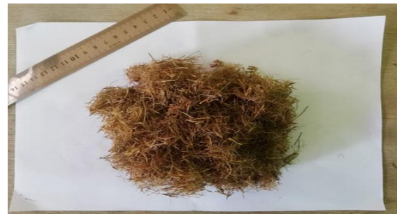
Fig.3: Polypropylene Fibers (PF). Fig.4: Date Palm Fibers (DPF) after Treatment.
