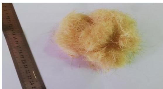
Fig.5: Flax Fibers (FF) after Treatment. Fig. 6: Date Palm Spikelet Fibers (DPSF)
