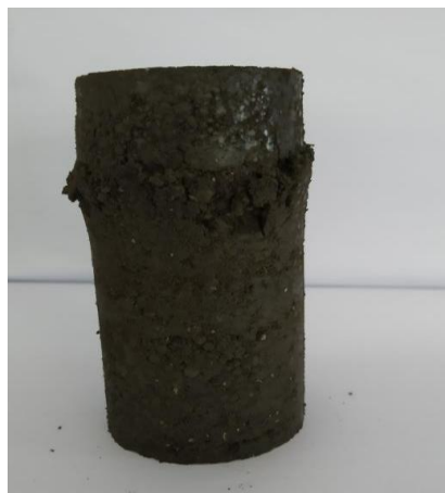
Figure 4.18 Failure characteristic of 1.5% xanthan gum treated soil
