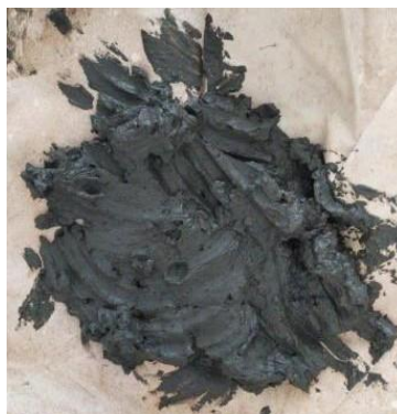
Figure 3.1 dredged marine soil
