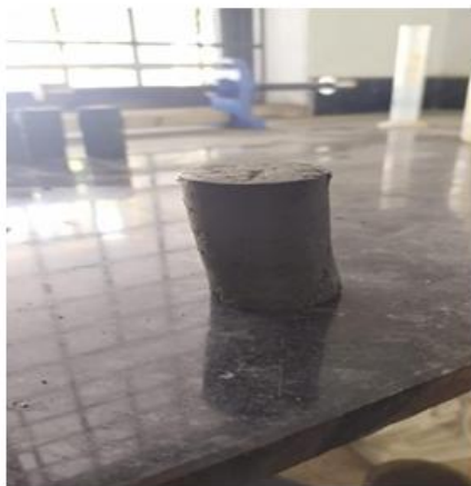
Figure 3.5 failure characteristics of raw soil
