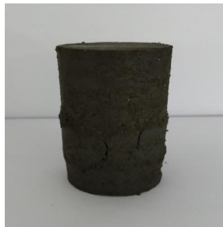
Figure 4.20 Failure characteristic of 0.3% chitosan treated soil
