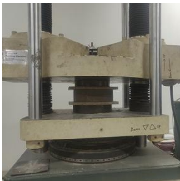
Fig 11: Placed CSEB in UTM machine
