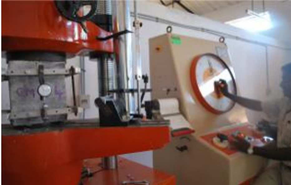
Figure 5 Compression Testing of Brick Masonry
