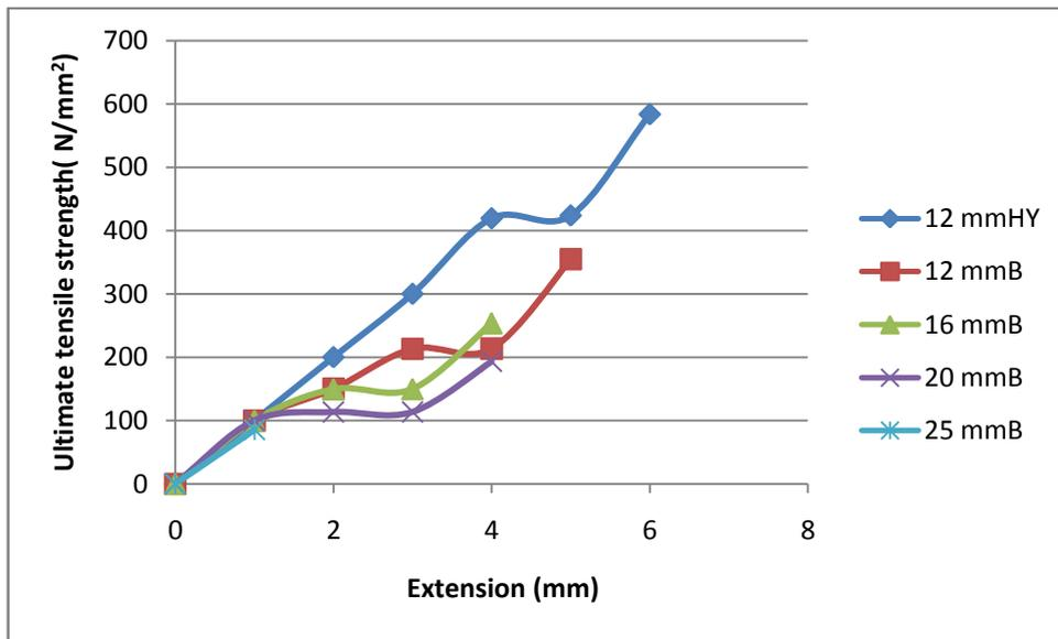
**Fig. 2:** Ultimate tensile strength vs Extension curve of Steel and bamboo rods
