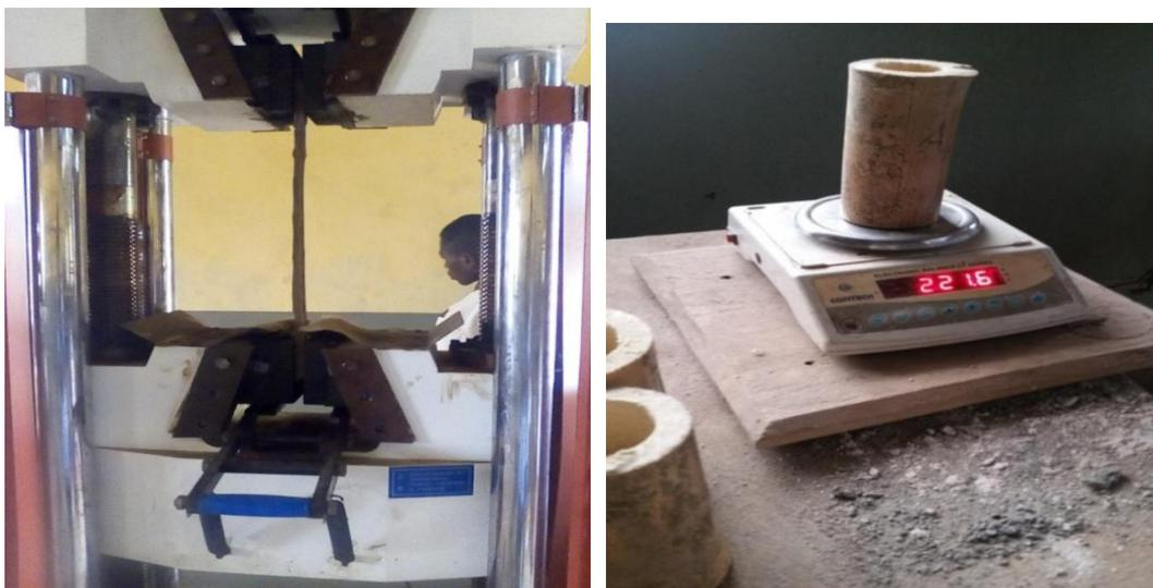
**Plate 3:** Tensile strength of splint bamboo **Plate 4:** Weighing Bamboo for Compression
