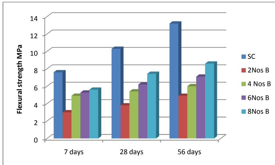
**Fig.6:** Flexural strength of 25 mm width bamboo
