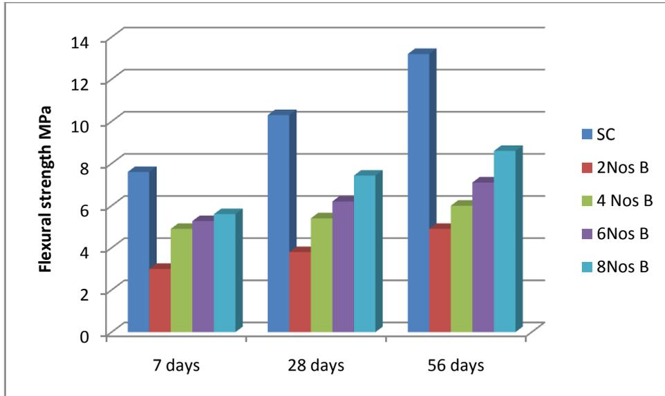
Fig. 4: Flexural strength of 16 mm width bamboo
