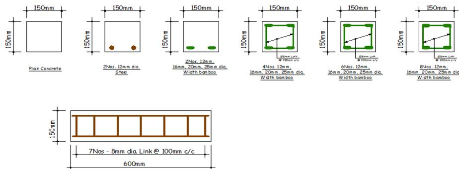
Fig. 1 Section Through Reinforced Concrete Beam (Plain, Steel and Bamboos)
