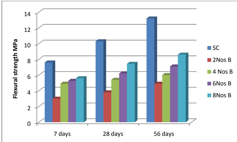
Fig. 3: Flexural strength of 12 mm width bamboo-reinforced concrete
