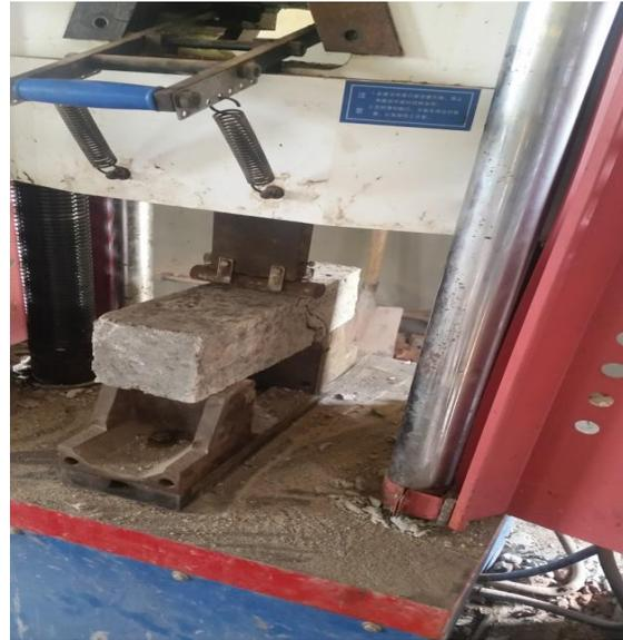
Plate 7: Arrangement of Reinforcement Plate 8: Flexural strength test of concrete beam
