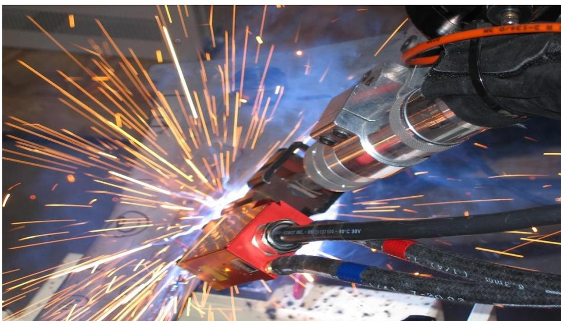
**Figure 7: Robotic Welding using Servo-Robot Laser Vision**
