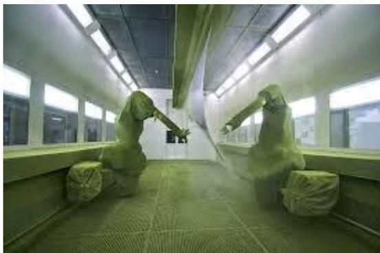
**Figure5b:** trajectory painting robots
