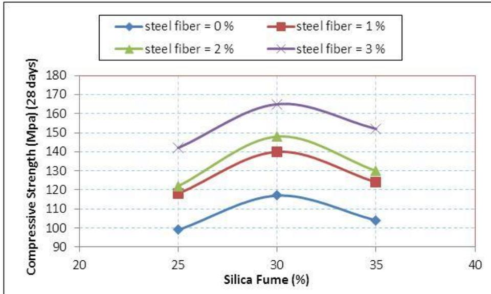
Figure 24: Impact of SF content on RPC compressive strength containing different ratio of SF at 28 days
