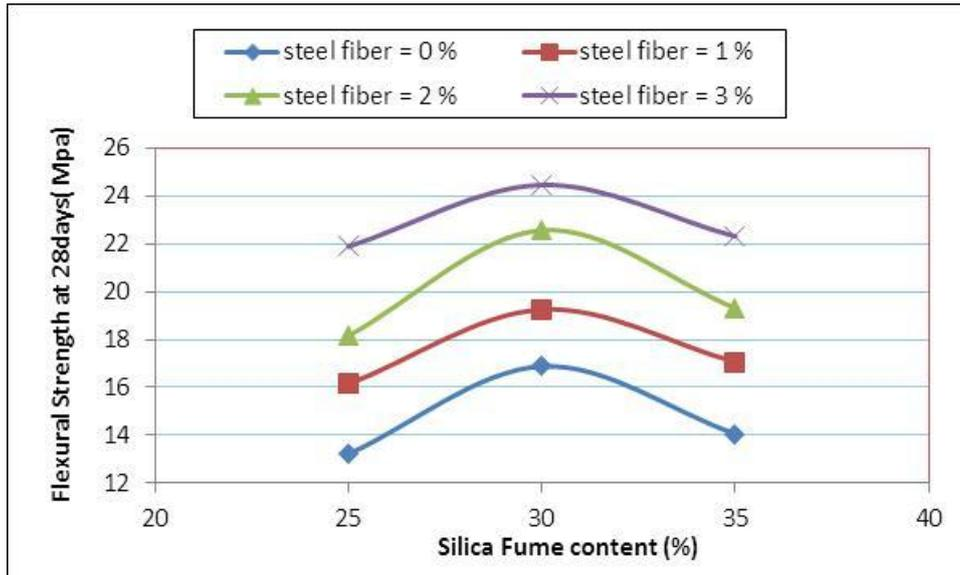
Figure 39: Influence of SF and steel fibers on RPC flexural strength with various percentage of steel fiber at 28days
