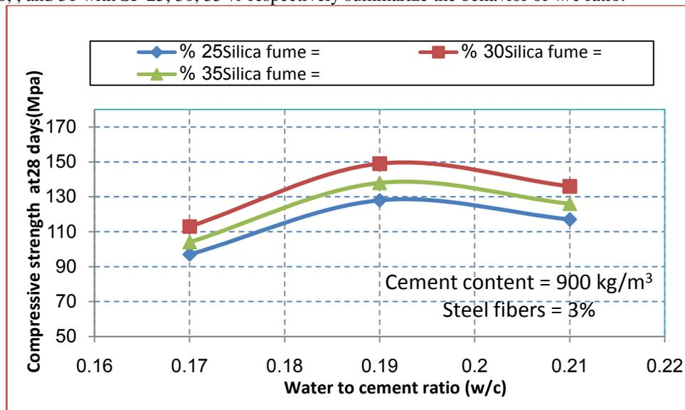
Figure 30 Effect of water to cement ratios (w/c) on Compressive Strength.
