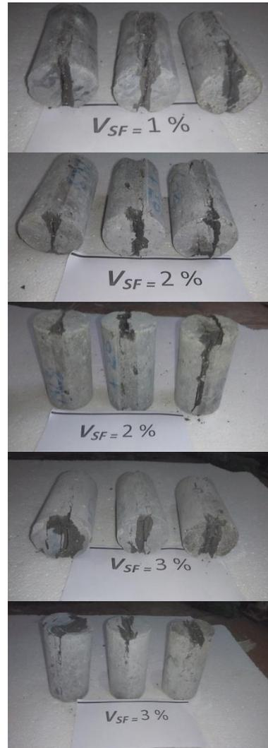
Figure 37: Effect of steel fibers content on shape of specimen's failure in Splitting tensile strength test
