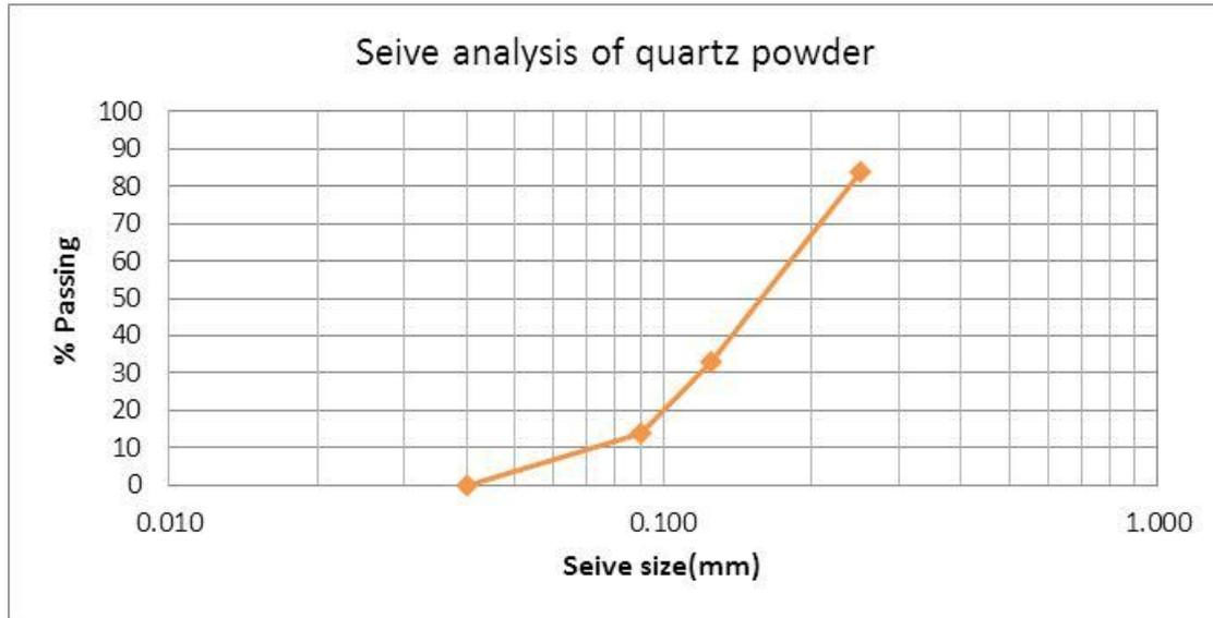
Figure 6: Grading of quartz powder.
