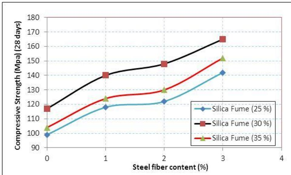
Figure 27: Impact of steel fibers on RPC compressive strength containing different ratio of silica fume at 28 days
