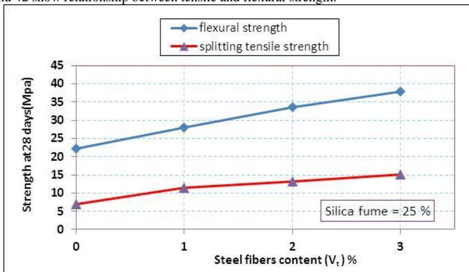
Figure 41: Relationship between tensile and flexural strength
