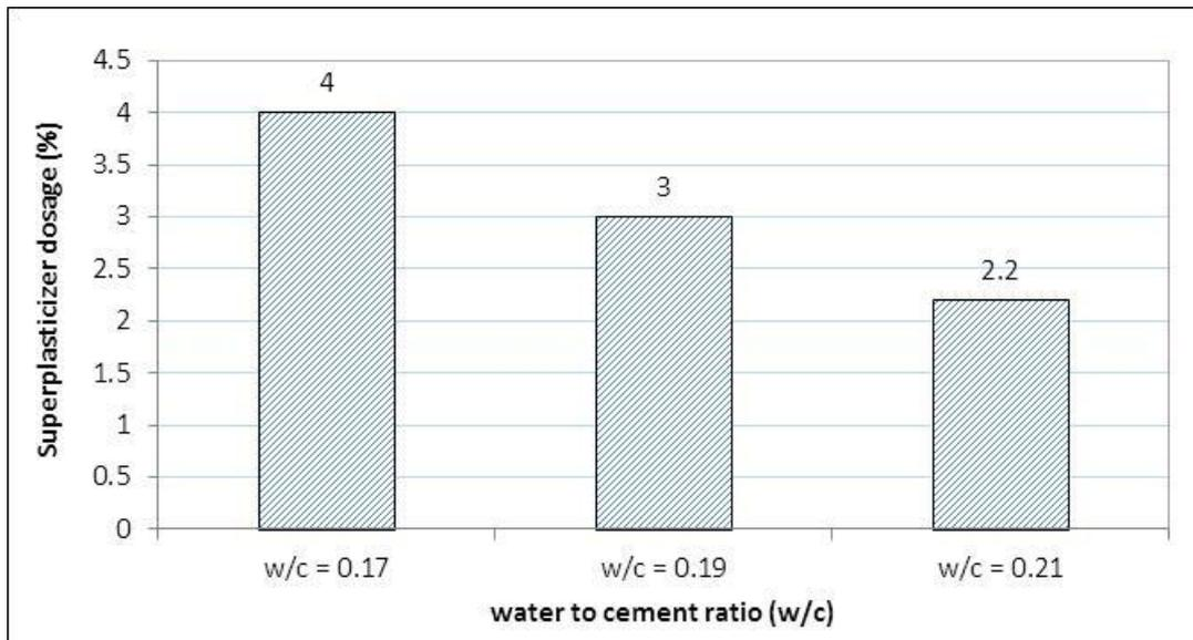
Figure 17: Correlation between w/c ratios and superplasticizers dosage
