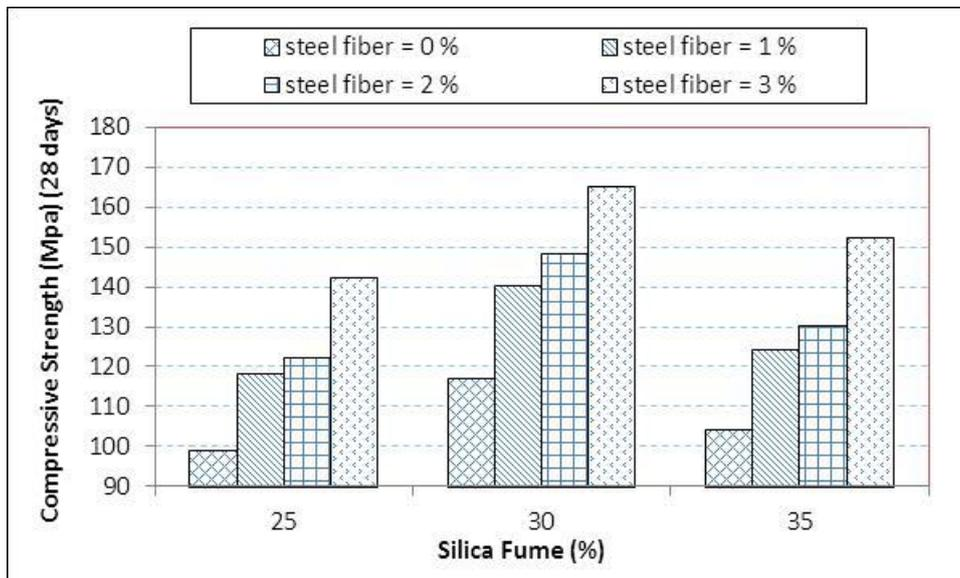
Figure 25: Impact of SF percentage on RPC compressive strength containing different ratio of steel fibers at 28 days
