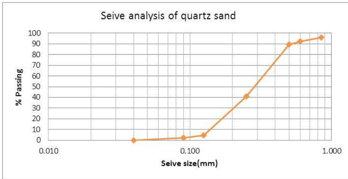
Figure Figure4: Grading of quartz sand.
