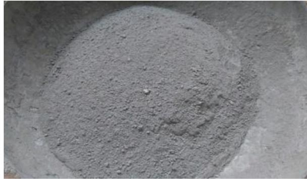
**Figure 10: RPC mix after dry mixing**
