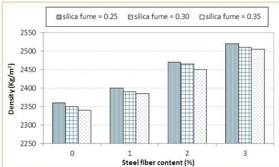
Figure 21: Impact of SF amount on RPC density with various contents of SF
