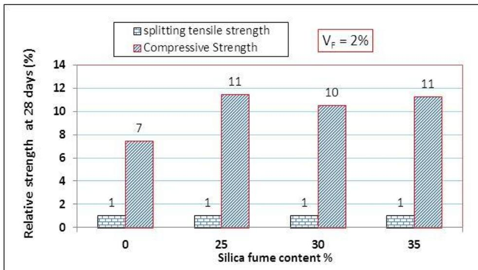
Figure 36: Relative compressive and splitting tensile strength with steel fiber (2%)
