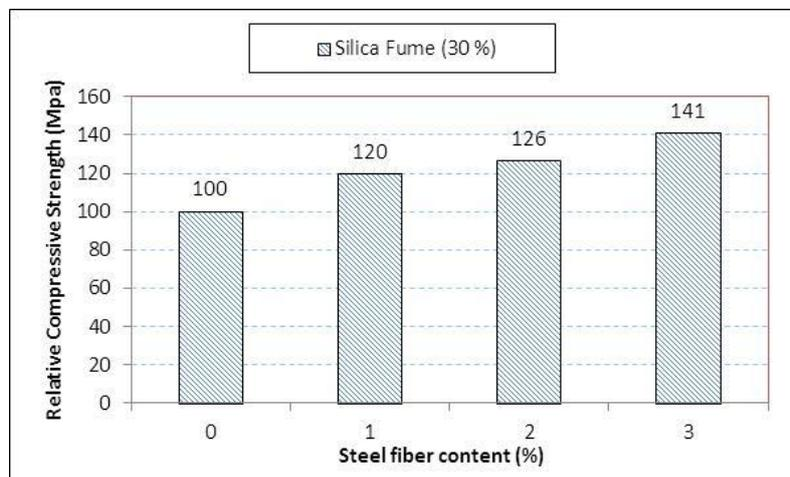
Figure 29: Influence steel fibers on Relative compressive strength of RPC having SF (30%)
