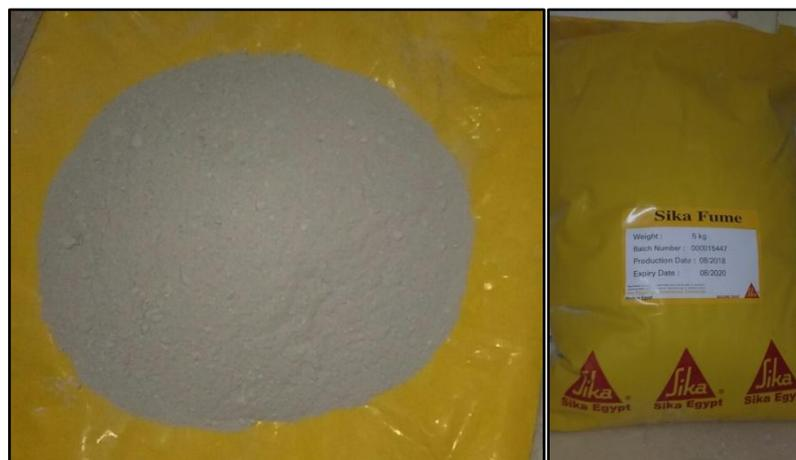
**Figure 2: Silica Fume used in mixtures**
