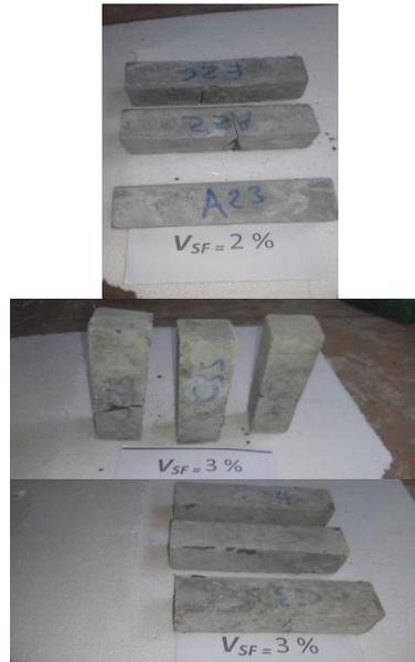
Figure 40: Impact of steel fibers percentage on shape of specimen failure in flexural strength test
