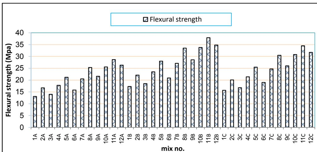
Figure 38: Results of Flexural strength of different mixes
