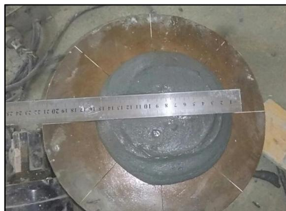
**Figure 16: Flow table test after working samples**
