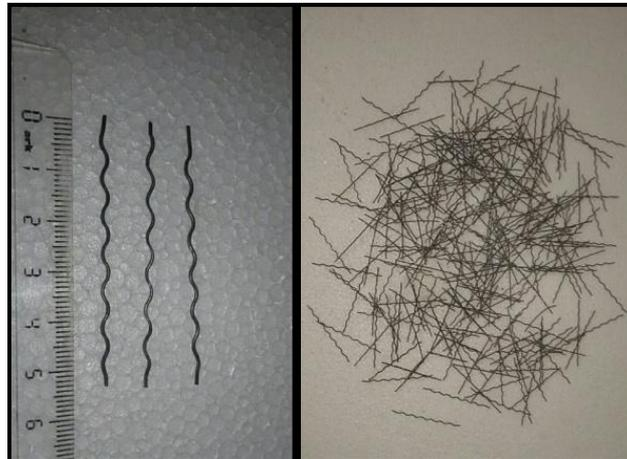
**Figure 8: steel fibers before cutting**
