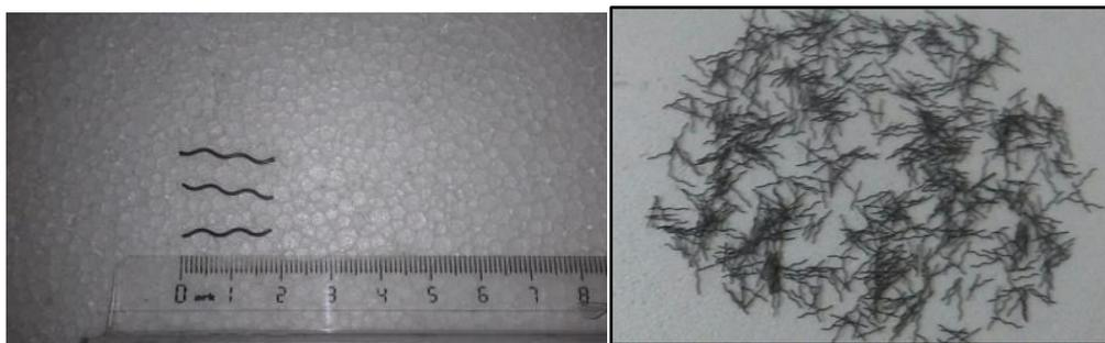
**Figure 9: Steel fibers after cutting into three parts**
