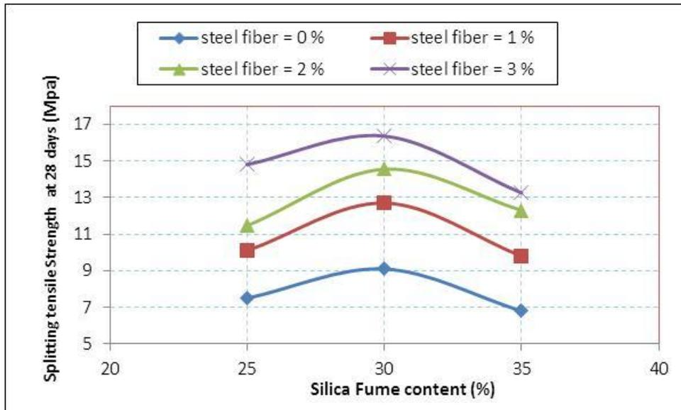
Figure 33: Influence of SF and steel fibers on tensile with various percentage of steel fiber at 28 days
