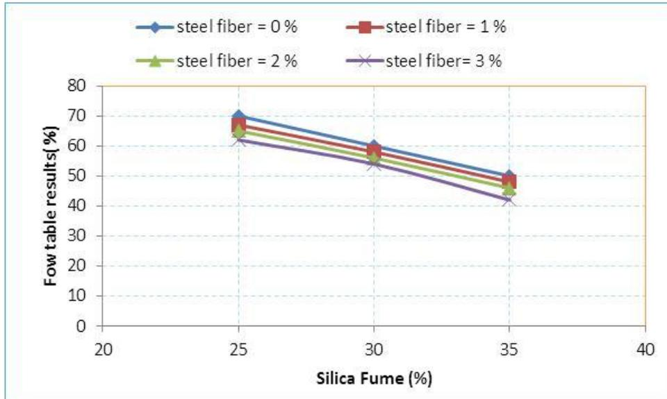
Figure 19: Influence of SF and steel fibers on flow table test results
