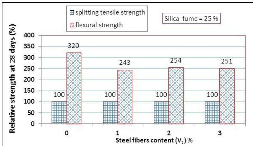
Figure 42: Relative relationship between tensile and flexural
