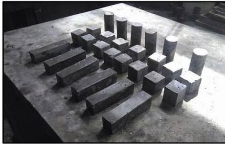
**Figure 14: Concrete specimens after casting**
