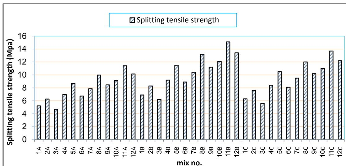
Figure 32: Results of splitting tensile strength of different mixes
