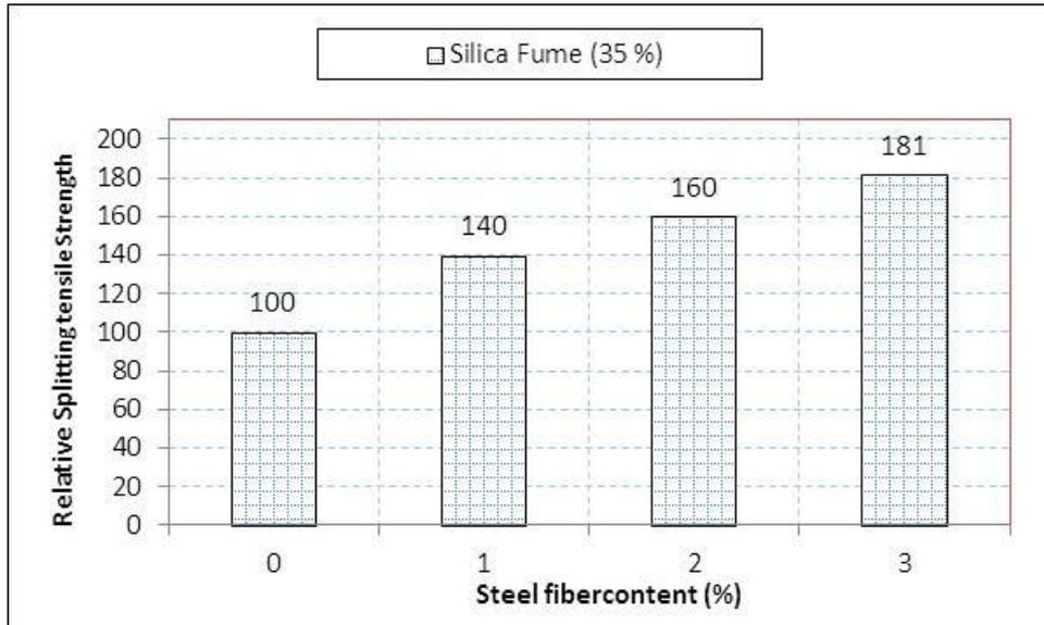
Figure 35: Relative tensile to S<sub>t</sub>F with silica fume (35%)
