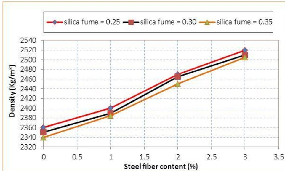
Figure 22: Impact of steel fibers content on RPC density with different contents of silica fume
