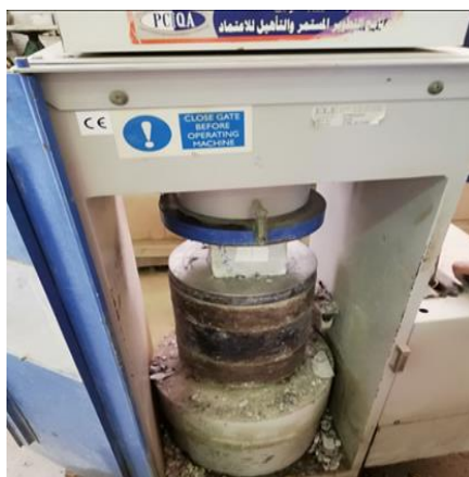
Fig. 4: Cube (10 × 10 ×10 cm) during Compressive Strength test
