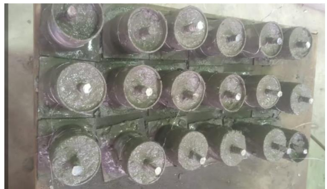
Fig. 4: Cylinders (70 ×100 mm) During Casting
