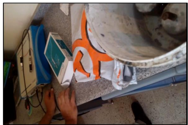
Fig. 5: Cylinder (7 × 10 cm) During Measuring Corrosion
