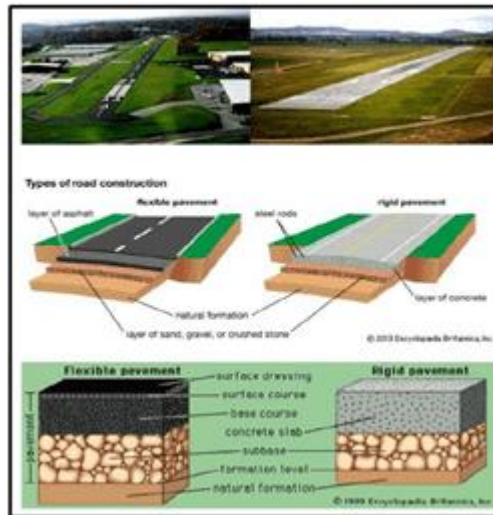
Figure 3. Difference between Rigid Pavement and Flexible Pavement
