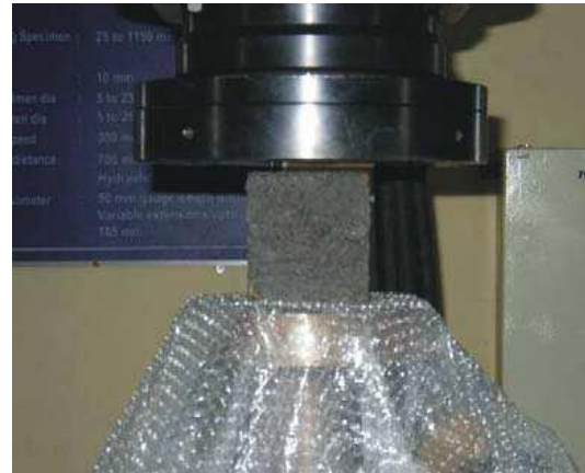
Figure 4.2 (b): Testing of cubes in UTM Table 4.1:
