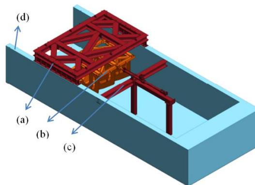
**Fig. 4 Conceptual design of a piston-type displacer: (a) stationary frame assembly; (b) moving frame assembly; (c) actuator frame assembly; and (d) flume wall**
