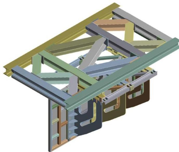
**Fig 7. Retracted position of the displacer assembly**
