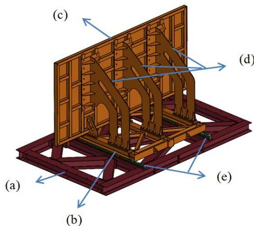
**Fig. 5. Details of the wave board assembly in the upright position: (a) stationary frame assembly; (b) moving frame assembly; (c) wave paddle; (d) stiffener plates; and (e) LM Guide rails**
