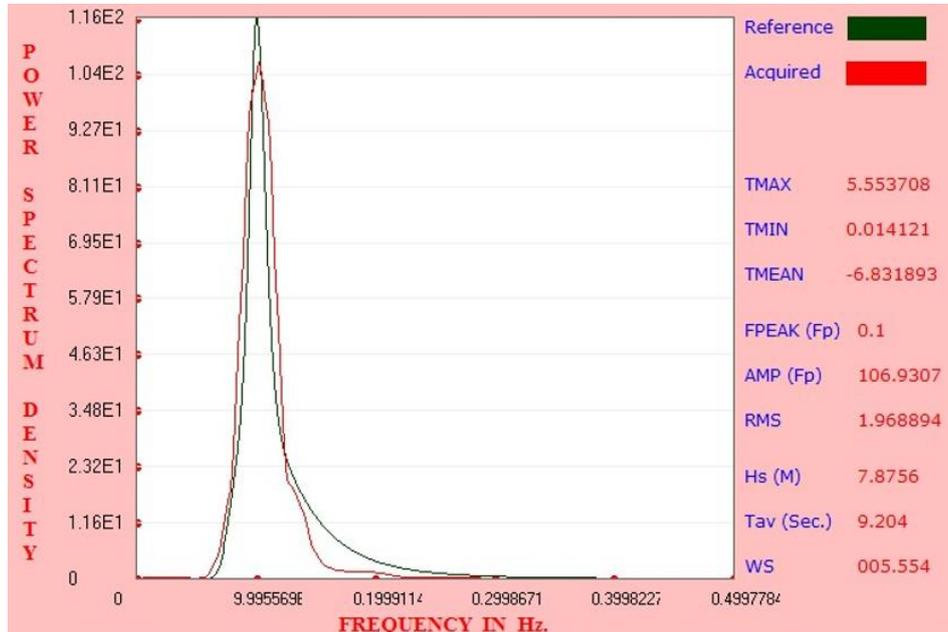
**Fig. 9 Matching of the frequency spectra of the waves generated by a piston-type wavemaker with a wave flume of length 120 m and a water level of 0.8 m with the target JOHNSWAP spectra; the model scale is 1:56, reference Hs=7.75 m, acquired Hs = 7.8756 m (the percentage of spectrum match with respect to Hs = 98.4% with a percentage error of 1.6%)**
