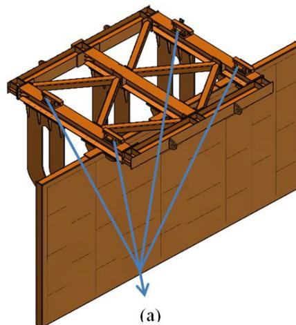
**Fig 6. Details of moving frame assembly with the paddle, stiffener plates and LM Guide: (a) LM Guide**
