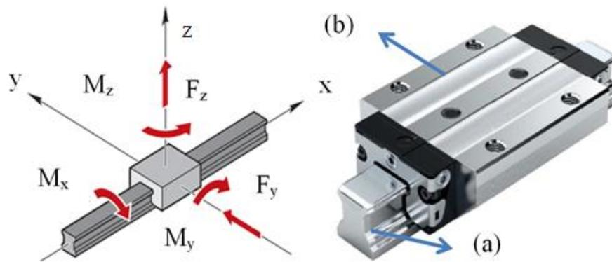
**Fig 8. Details of linear motion guideways: (a) Guide rail (b) Runner block, Travel speed:  $V_{max}=5$  m/s,  $F_y=190$  KN,  $F_z=111$  KN**
