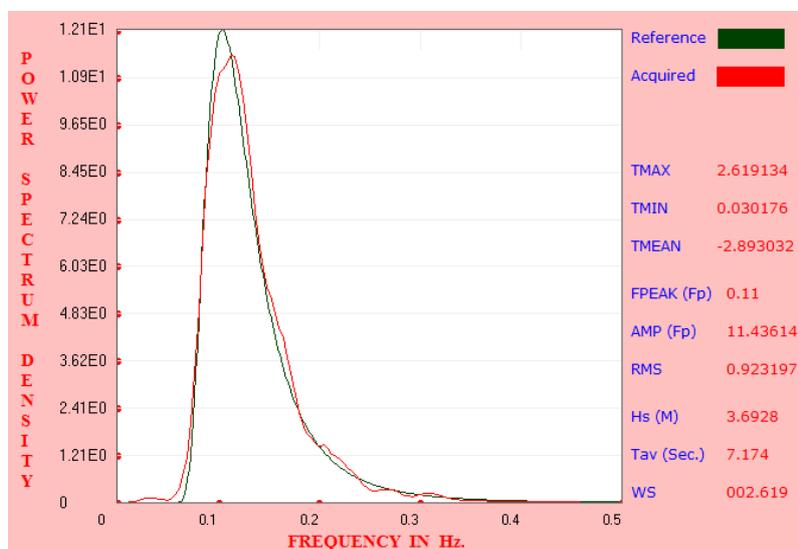
**Fig. 10 Matching of the frequency spectra of the waves generated by a piston-type wavemaker with a wave flume of length 120 m and a water level of 1 m with the target Pierson-Moskowitz (PM) spectra; the model scale is 1:25, reference Hs =3.75 m, acquired Hs = 3.6928 m (the percentage of spectrum match with respect to Hs = 98.4% with a percentage error of 1.6%)**
