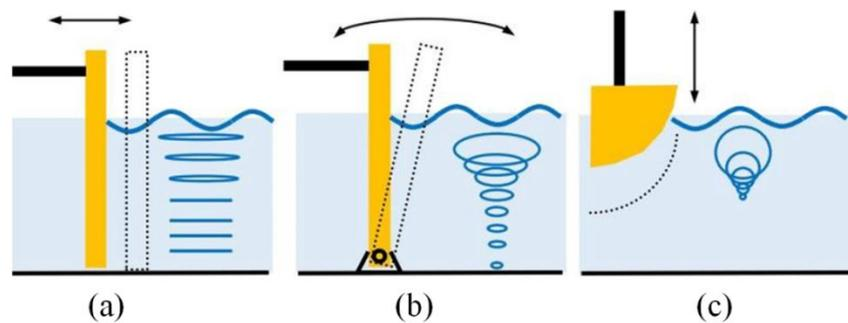
**Fig. 1 Schematics of the figures: (a) piston-type (linear); (b) flap-type; (c) plunger-type**
