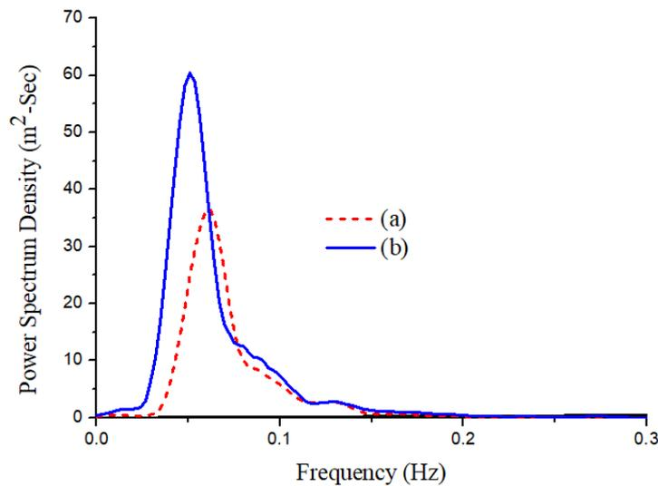
**Fig. 12** Experimental results of the target Pierson-Moskowitz (PM) spectra with different significant wave heights (Hs), and a water depth of 1.1 m in the flume; at a model scale of 1:25: (a) Hs= 0.15 m in the model generated using Pierson-Moskowitz (PM) spectra. (b) Hs= 0.27 m in the model generated using Pierson-Moskowitz (PM) spectra.
