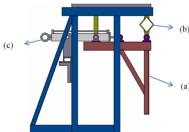
**Fig. 2 Schematics of a typical top-hinged suspended pendulum-type wave displacer at the CWPRS: (a) Wave board; (b) Diamond-beam; and (c) Actuator**
