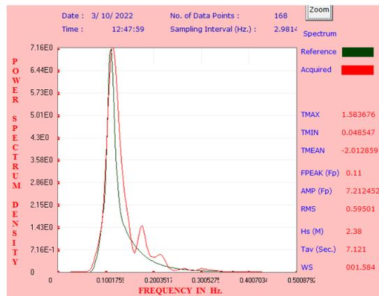
**Fig. 3 Generation of the wave spectrum by using a top hinged flap type wavemaker with a passive wave absorber at the CWPRS**
